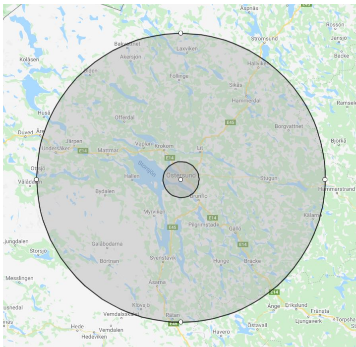
Figure 2: Theoretical serviceable range for (small) urban drones and (large) inter-city drones with the longest range
