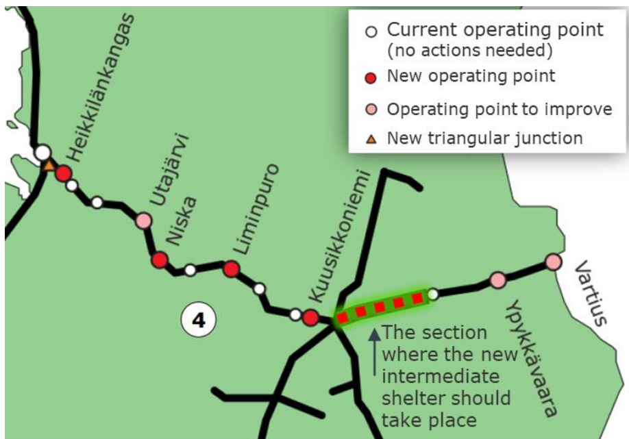
Figure 30: Distance between safety points Arola-Kontiomäki interval is really long (+40 km). It is the largest infrastructural bottleneck in Vartius traffic. (Source: VR Group)
