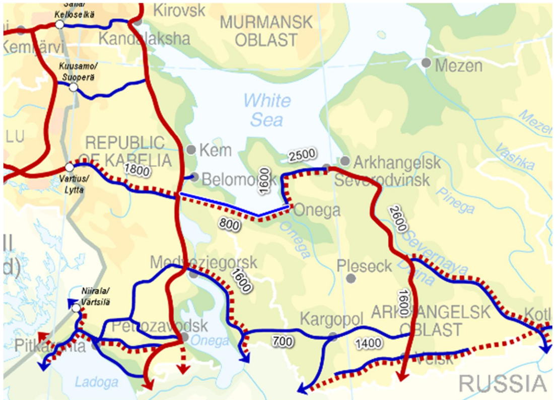
Picture. Forecast of the distribution of current traffic volumes on the main road network including the new road Vartius - Arkhangelsk, AADT 2020, vehicles/day. (Modified from the Source: Barents Link Corridor- report, Joint Authority of Kainuu Region, 2007)
