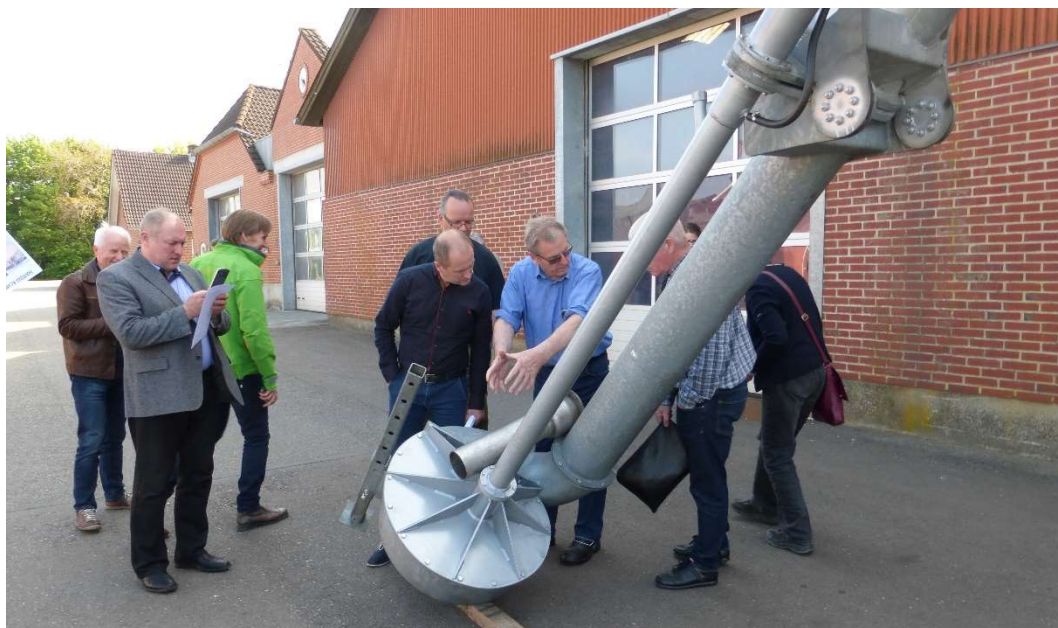
HARSØ equipment for in-tank acidification is being demonstrated to the tour participants.
