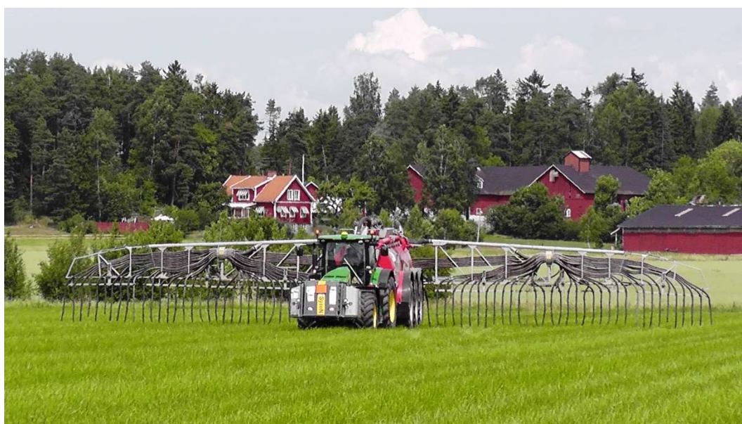
Br. Göranssons testing their in-field slurry acidification equipment.
