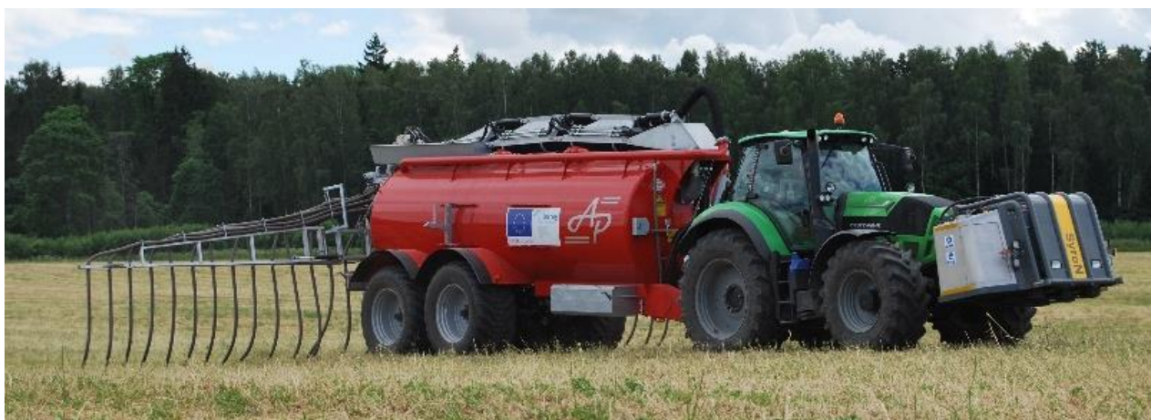
Figure: In-field SAT investment (SyreN) made by LUHS in Lithuania spreading acidified slurry on their experimental farm.
