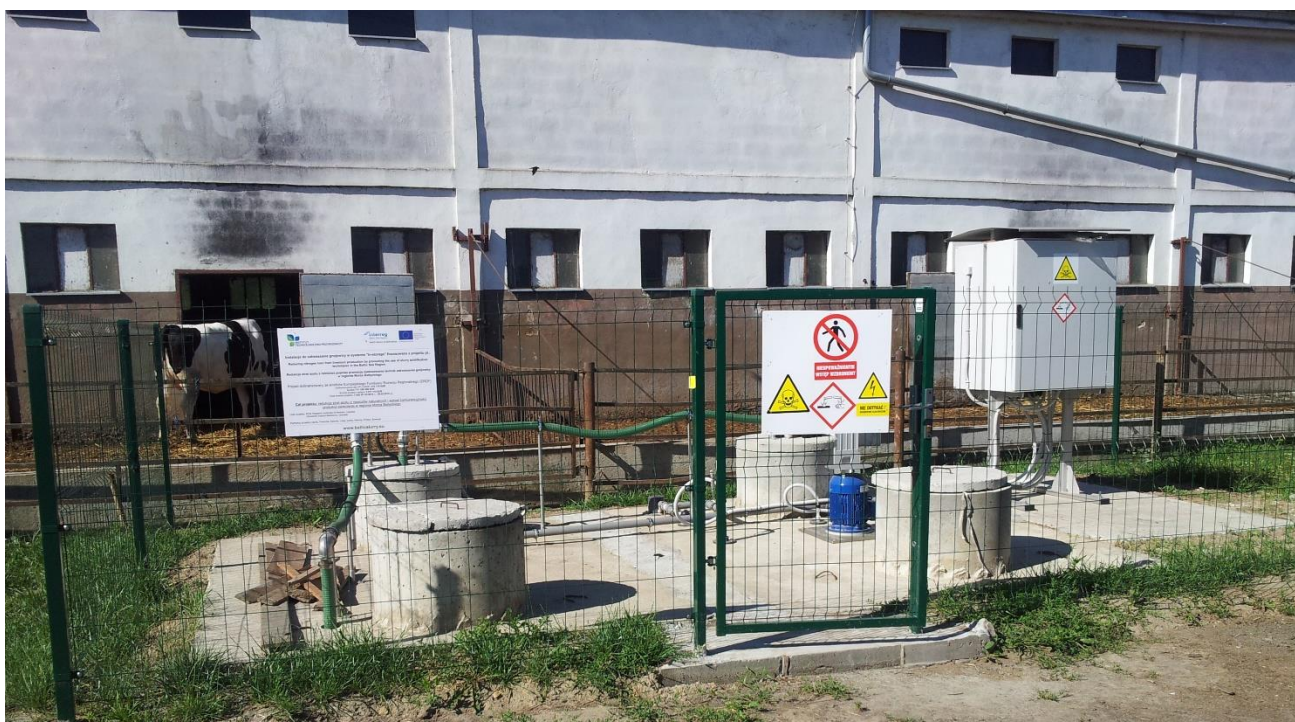
Figure: The small-scale In-storage SAT investment designed by ITP for experimental purposes at their Falenty field station.
