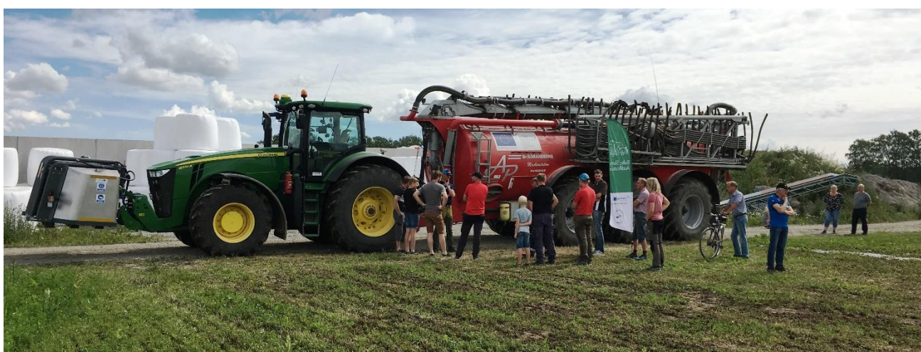
Figure: In-field SAT investment (SyreN) made by Br. Göransson on display at a demonstration in Sweden.
