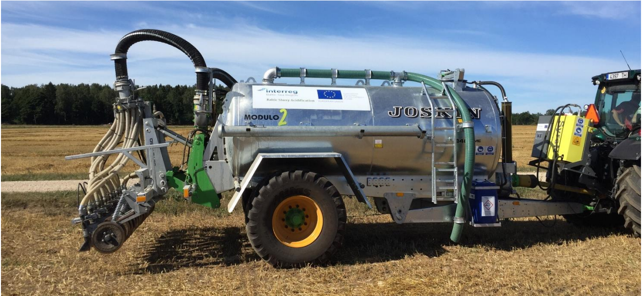
Figure: In-field SAT (SyreN mini) investment made by ECRI. The SyreN mini was produced specifically to work with smaller tankers for research purposes.
