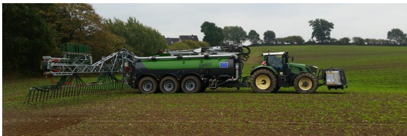
Figure: In-field SAT investment (SyreN) made by Blunk GmbH in Germany spreading acidified slurry during a demonstration outside of Kiel.
