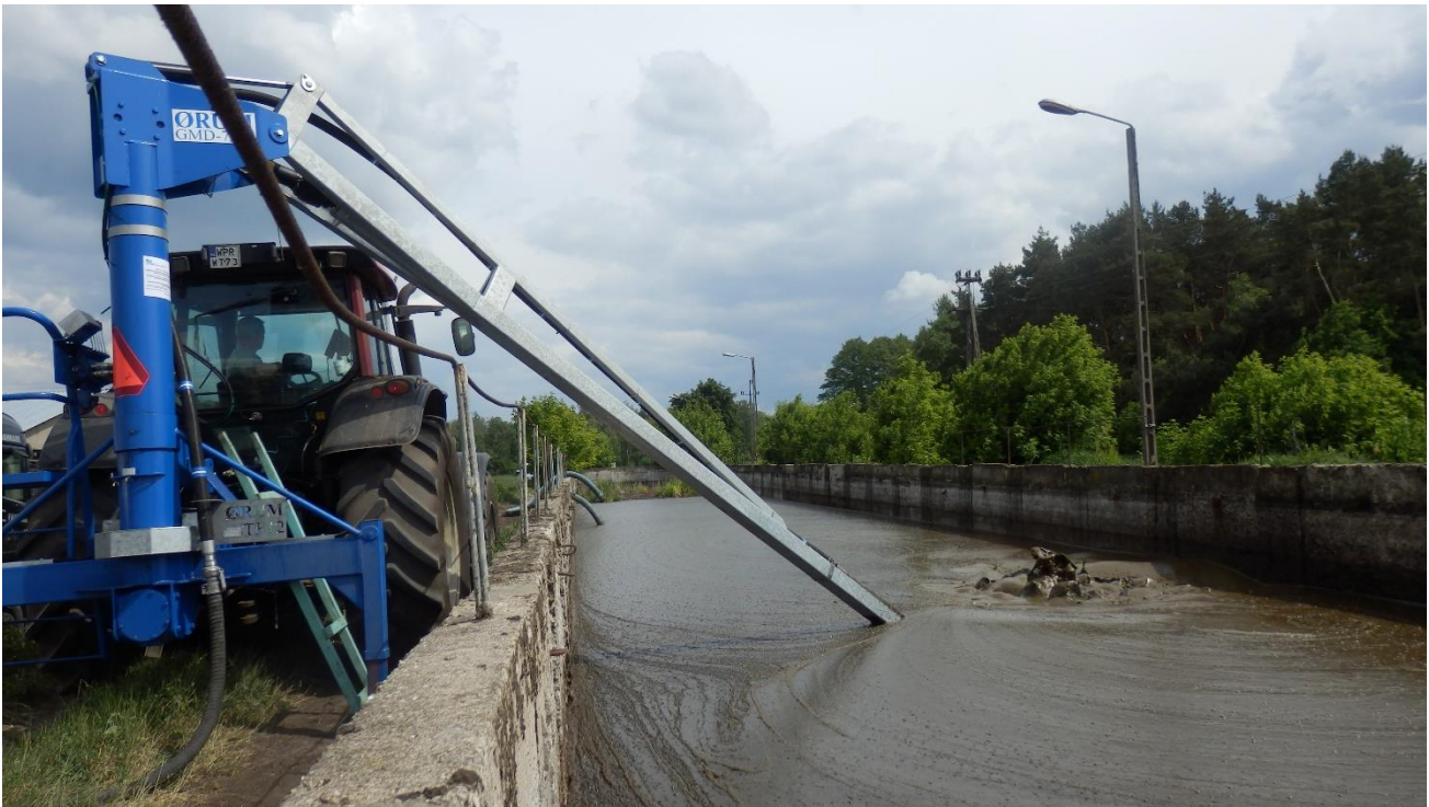
Figure: In-storage SAT investment (Ørum) made by ITP in Poland, here acidifying slurry at ITP's experimental farm in Biebrza.
