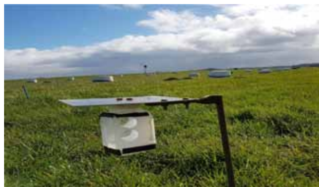
Figure 5. Used acid trap to capture volatile ammonium on a grassland plot (Source: Sebastian Neumann, LLUR).
