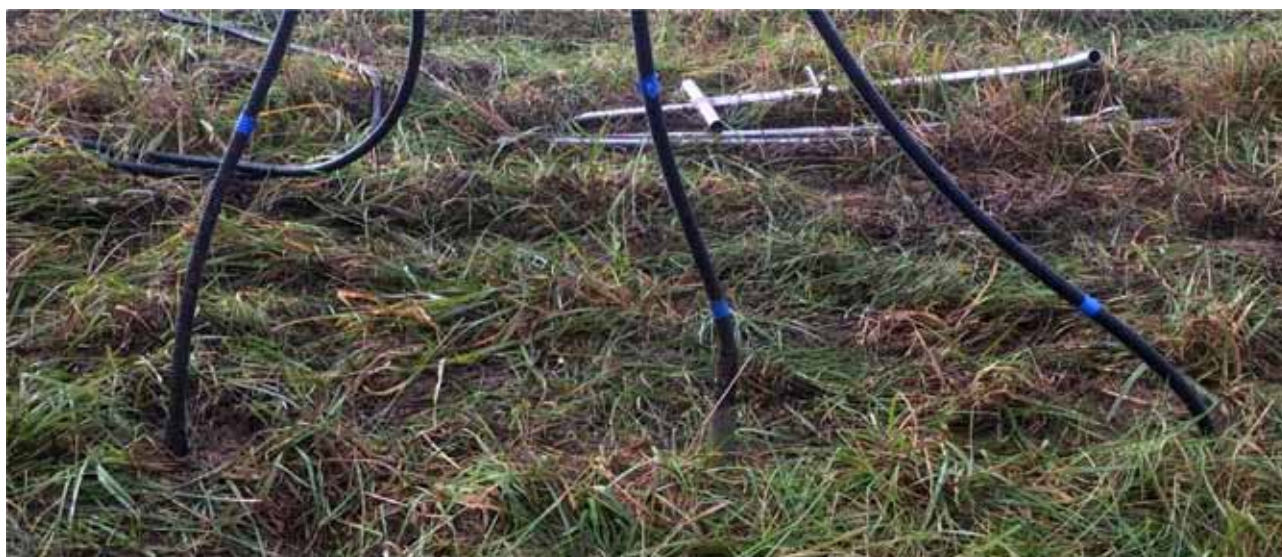
Figure 8. Sensors on cattle slurry (2) plot. From left: 15 cm sensor, 5 cm sensor and 25 cm sensor.
