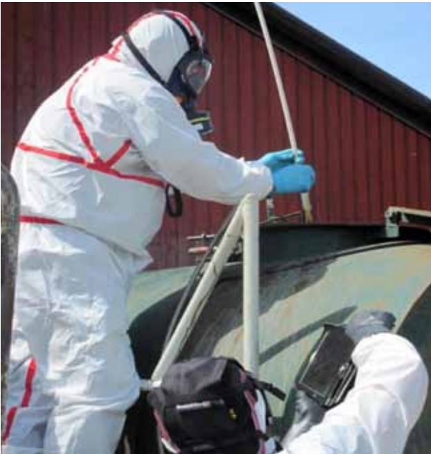
Figure 6. The slurry pH and temperature were measured several times by sinking the sensor into the sampling vessel. Photo: Gunnar Lundin
