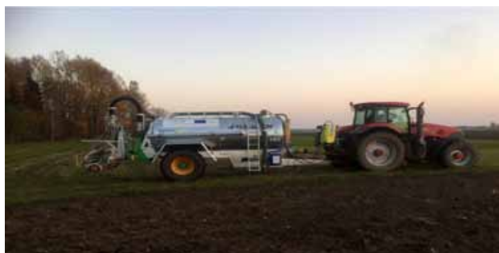
Figure 3. ECRI slurry spreader with SyreN in-field acidification system on demonstration trial field in Jõgeva, Estonia. Picture by Kalvi Tamm.
