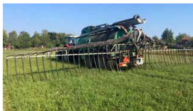
Figure 6. Irrigation of the experimental field on 17 th July. For this purpose, a slurry spreader equipped with trailing hoses was used. Photo: Anders Ringmar
