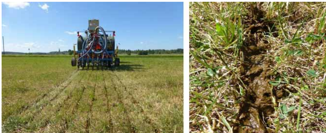
Figure 2. The experimental spreader placed slurry in bands on the ground. Spreading of untreated slurry. Photo: Gunnar Lundin
