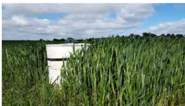
Figure 6. Measurement of nitrous oxide with the usage of extensions in wheat by the “closed chamber” technique (Source: Sebastian Neumann, LLUR).
