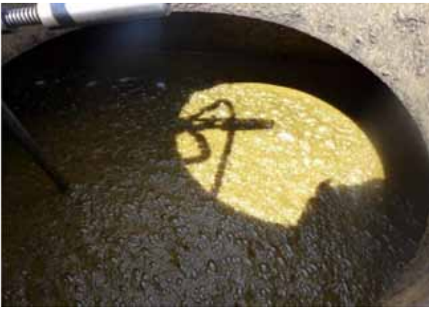
Figure 5. Extensive foaming occurred in the spreader tank while adding the acid, almost all the way to the top. The iron pipe used to add acid at the bottom of the tank can be seen on the left hand side of the picture. Photo: Lena Rodhe
