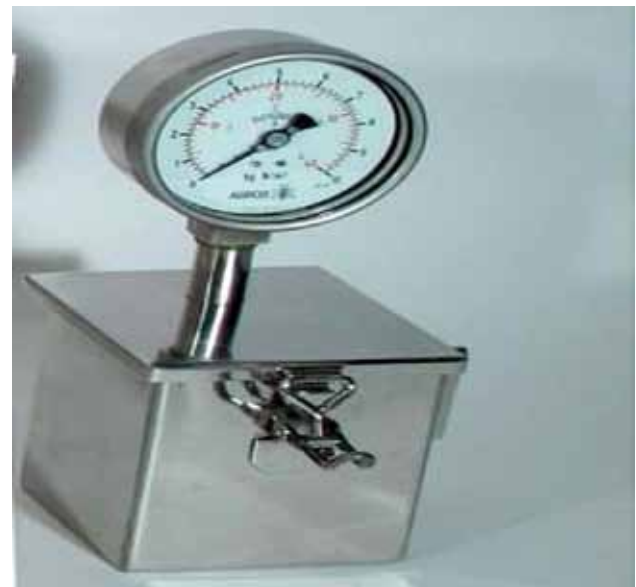
Figure 2. Nitrogen-meter “Agros”, used for quick analysis of ammonium-nitrogen content in field.
