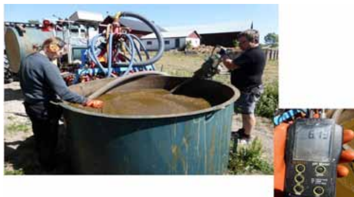
Figure 3. Stirring of acidified slurry and measuring of pH just before spreading. Photo: Gunnar Lundin
