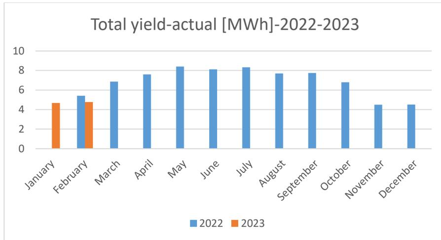
Fig.8 PV system yield (MWh) of year 2022-2023
