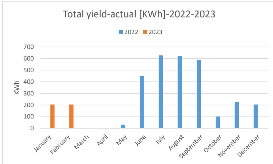
Fig.10 PV system yield (kWh)of year 2022-2023
