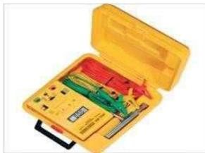
Digital Earth resistance test device
