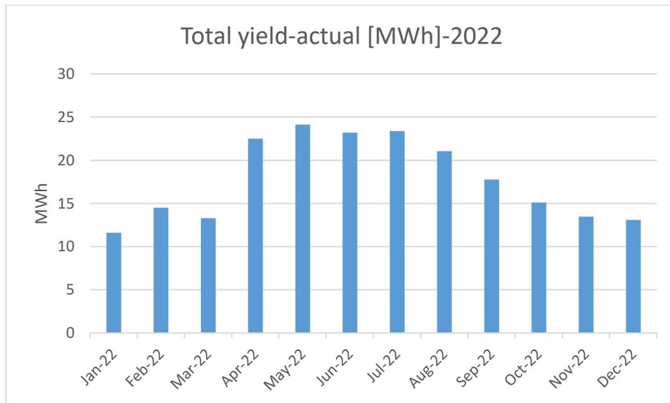
Fig.13 PV system yield of year 2022 -MWh
