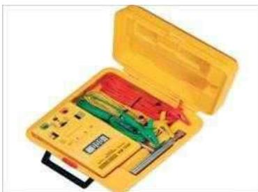
Digital Earth resistance test device
