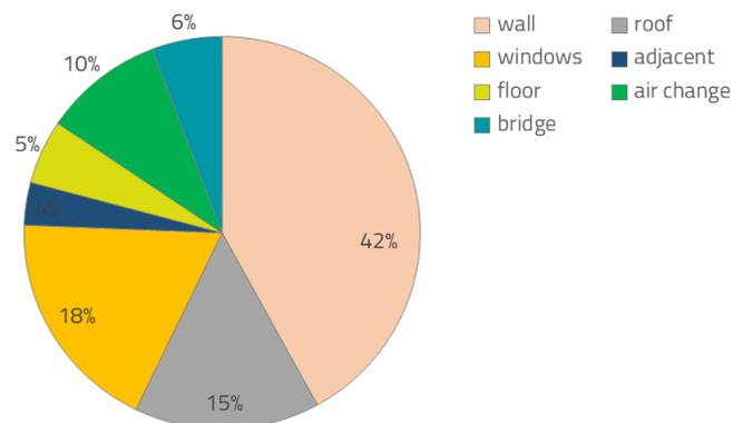
Therefore, the retrofitting process in this specific case must include a strong intervention on the envelope before considering plants and the integration of renewable energy sources. Depending on the overall area of each component, some evaluations have been carried out, aiming at the contribution for the amount of energy saving with the renovation of a mix of them. The results are reported in the table below with a target of -38% for heating consumption with a complete refurbishment.
