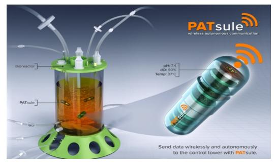
A scalable multi-parameter probe was developed during the H2020 AUTOSTEM project. The AUTOSTEM consortium developed an automated, sterile pipeline for large-scale production of therapeutic stem cells. The probe measured glucose, lactate and ammonia to support the culturing of stem cells in the bioreactor. The ultimate aim is to generate clinical quantities of high quality therapeutic stem cells at an affordable cost, thus enabling the routine clinical use of stem cell therapies in the future.
