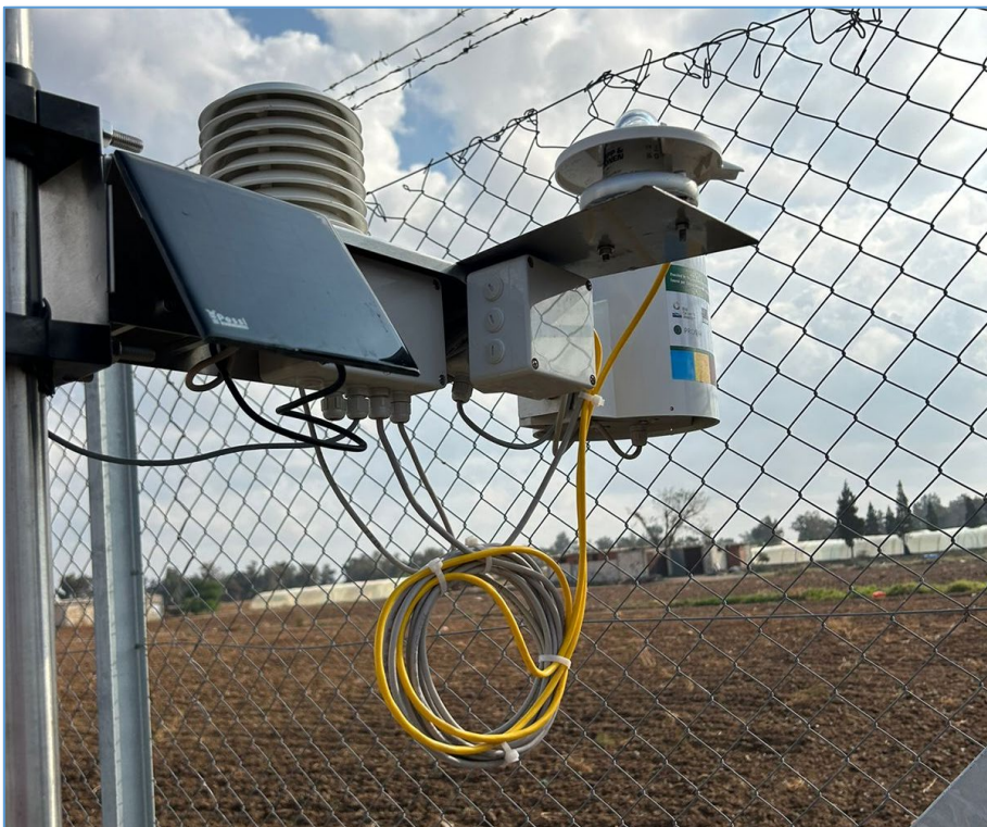
Photograph 6. Weather station used to inform the irrigation procedures based on real needs
