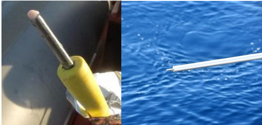
Figure 15-6. Arrow and tip (left) and tip on the aluminum pole (right) with the collected biopsy. (Photo ©UNISI).
