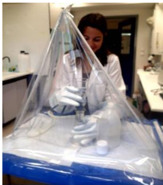
Figure 12-3. Filtration of digested sample in a glove box.
