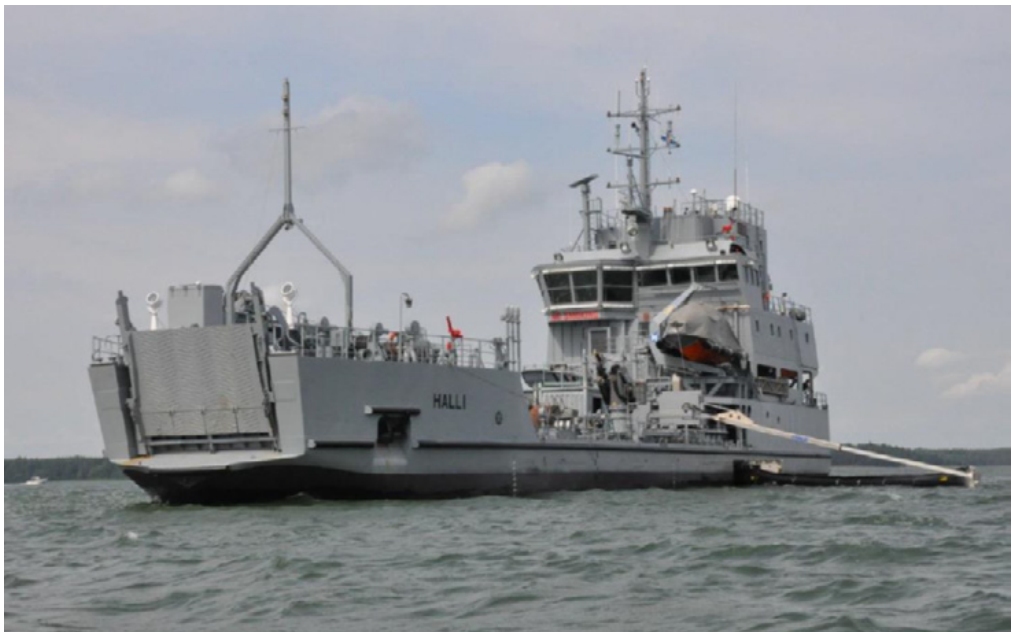
Figure 1. Finnish oil recovery ship HALLI with the inbuilt oil recovery system, inbuilt storage chamber for recovered oil and sweeping arms on both sides of the hull (reprinted from Häkkinen & Rytönen 2019).
