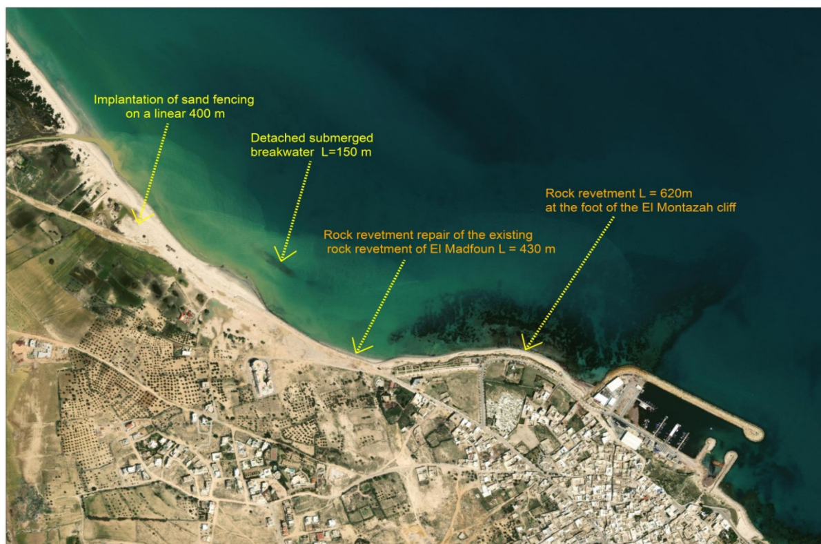
Figure 10. Protection works on the Hergla section, 2016
