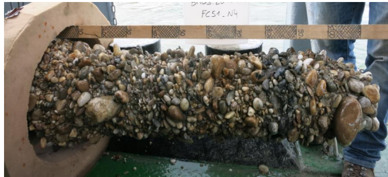
Figure 3.11: A freeze-core sample (photo: Philipp Gmeiner / BOKU)
