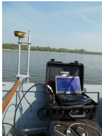
Figure 3.4: EcoTrac GPS receiver and a connected single beam echo sounder used for riverbed topography measurements in Hungary (Source: Debóra Varga-Lehofer)
