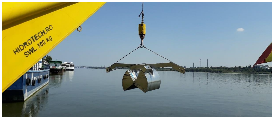
Figure 3.16: Grab sampler designed for bed material sampling (photo: Mravcova, VÚVH)
