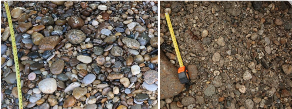
Figure 3.9: Volumetric samples from the Danube in Austria. Left picture: Surface; right picture: Subsurface (photos Philipp Gmeiner / BOKU)
