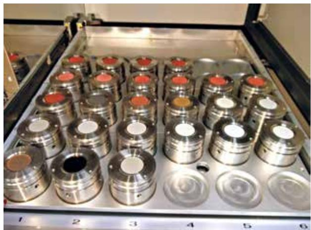
**Rigaku Primus II XRF spectrometer used in studies of the samples in the Institute of Ecology and Earth Sciences, University of Tartu**
