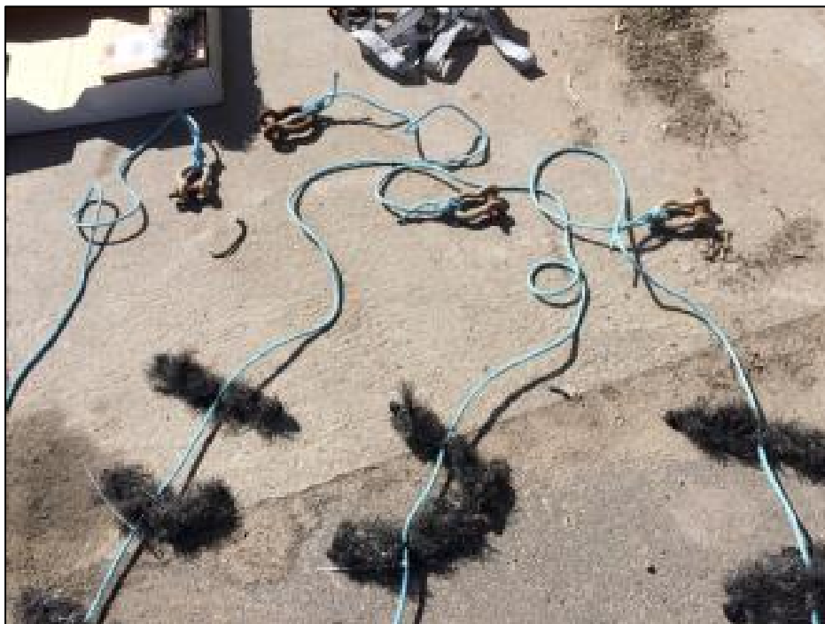
Picture 14. Ropes with triplicate pieces of fuzzy rope at 2-3m and at 5-6m ready to deploy at the Musholm site. The ropes were stretched with large shackles in the bottom.
