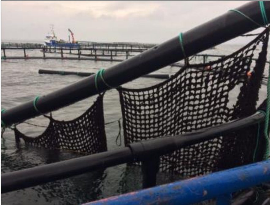
Picture 2. The test set up in 2016/2017, with two nets with different mesh sizes alongside each other, on a 10-meter PE tube.
