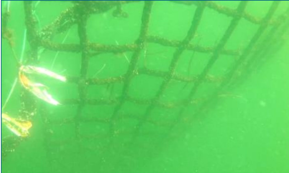
Picture 11. Depth study reaching down to 13 m depth with Smartfarm net (mesh size 150 x 150 mm).
