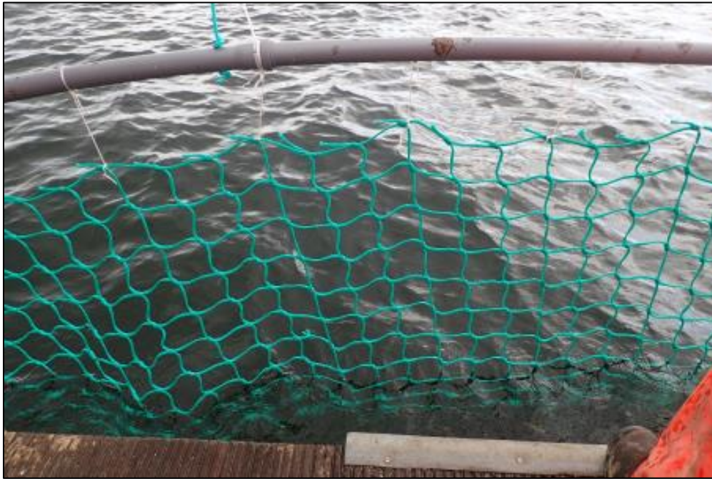
Picture 9. Set up with 100 x 100 mm mesh size trawl net in 2018/2019. Deployment the 4 th of June 2018.
