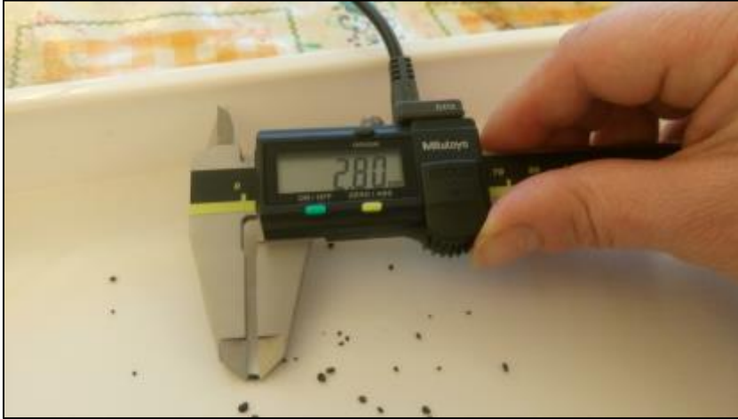
Picture 18. Working process with an electronic caliper, measuring very small mussel lengths.
