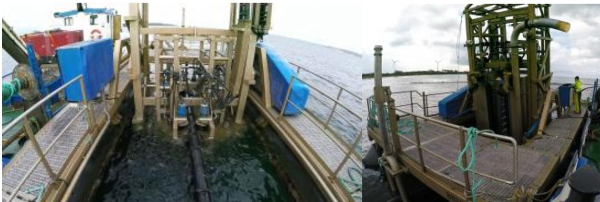
Figure 17: Harvest of a net farm (Musholm), using a UW harvester.
