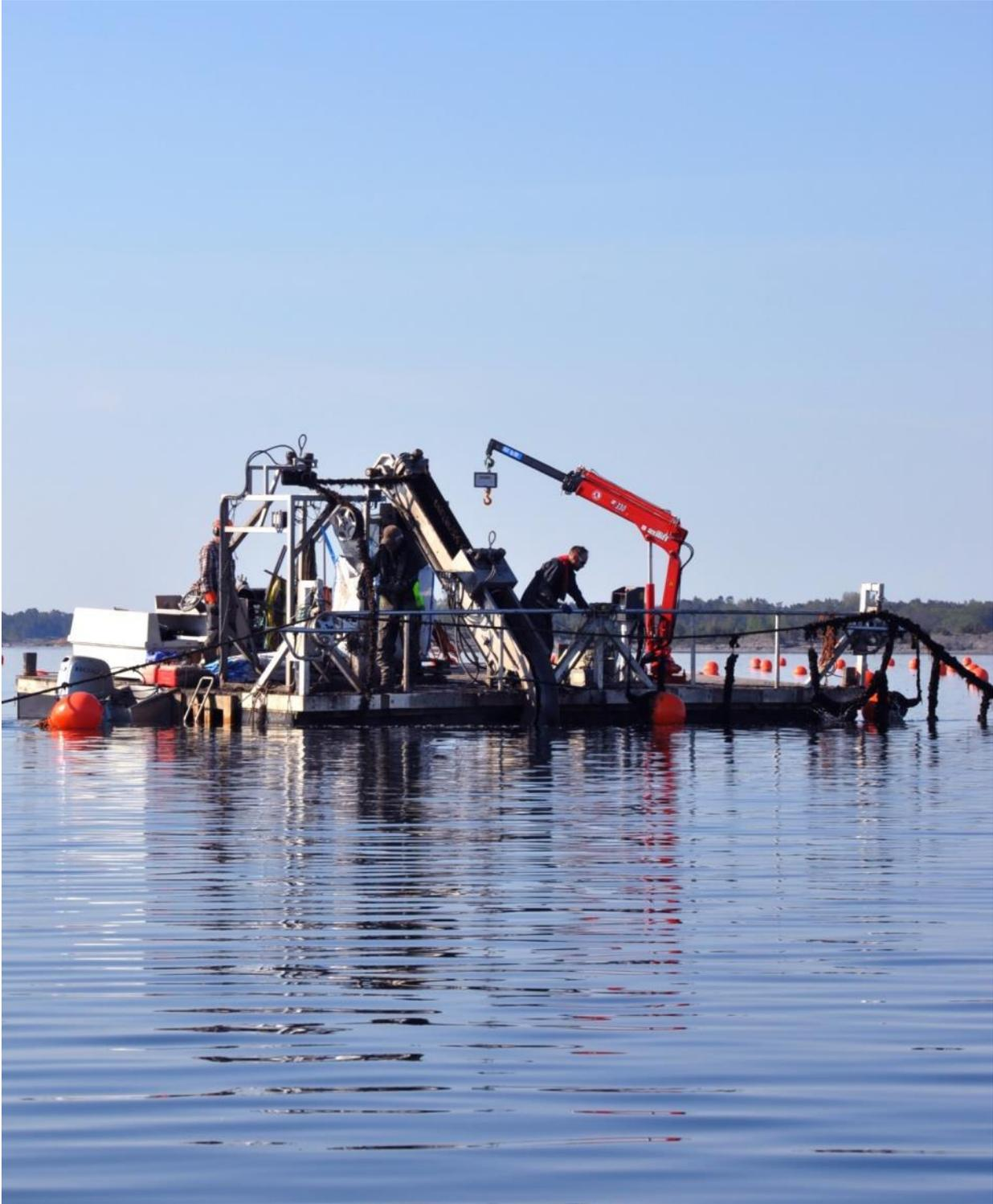
Figure 19: Harvest of long-line farm (St. Anna), using a conveyer belt to lift up the longline on a harvest platform and a scraper to clean the mussels from the substrate.
