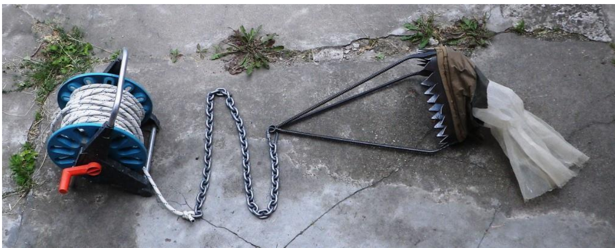
Figure 2: Bottom dredge with chain and rope for macroinvertebrate sampling
