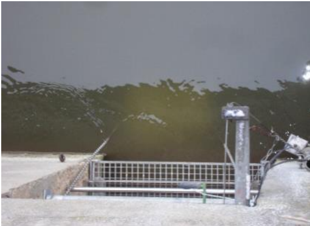
Figure 3: Exposition by means of stainless steel chains at a weir.
