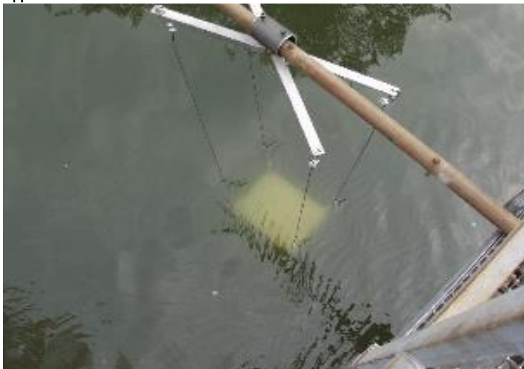
Figure 2: Exposition by means of stainless steel ropes from a bridge.
