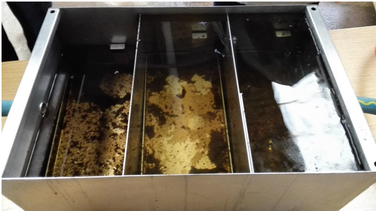
Figure 6: Open SB (stationary version) after weeks of sampling the effluent in a WWTP (Berlin).
