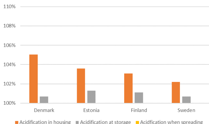
Figure 9. Increased of total nitrous oxide emissions from slurry when acidifying slurry in housing, storage or when spreading compared to reference, no acidification.
