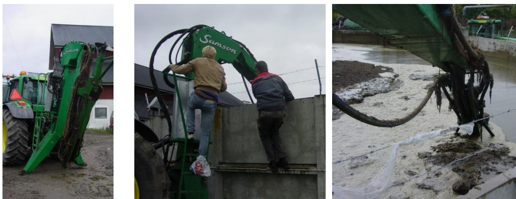
Figure 2-39. Use of a separate tractor driven mixer to mix in the straw crust just before spreading.
