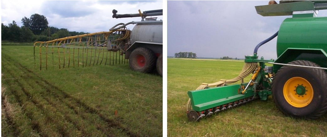
Figure 2-41. Band spreading is the dominating spreading technology in Sweden (left), but some slurry is spread also with injectors (right).
