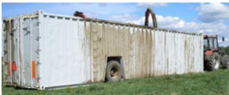
Figure 2-16. Mobile buffer tank for slurry placed in field.
