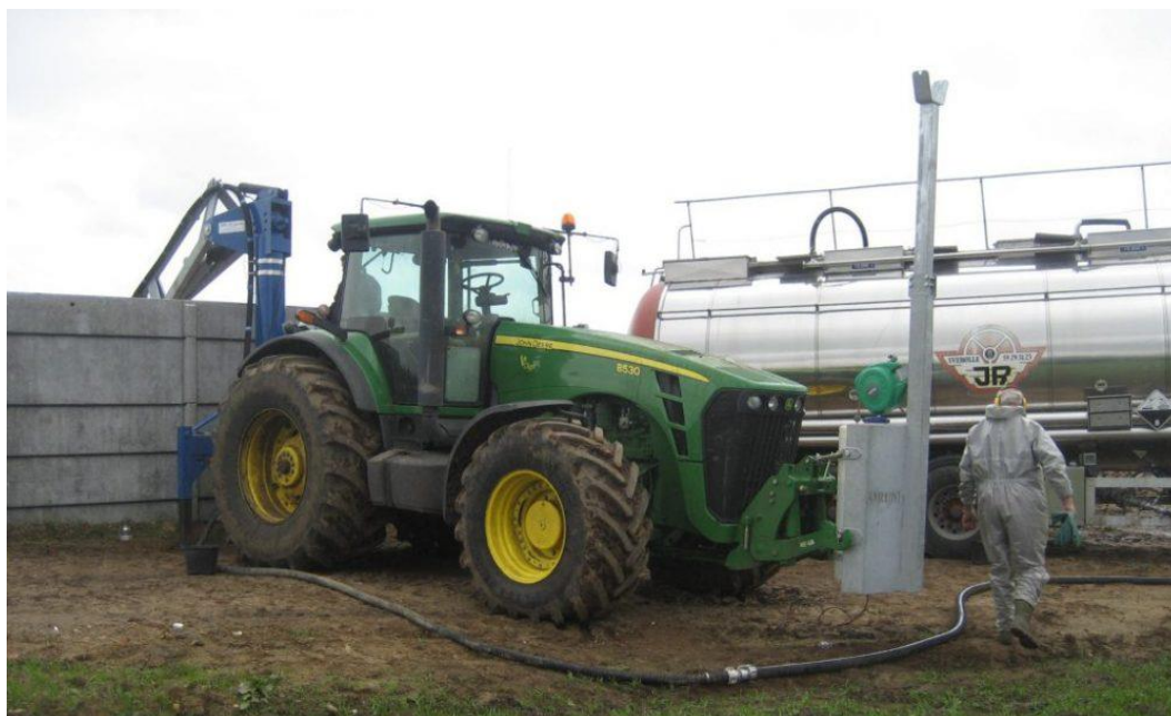
Figure 4.6. The Ørum SAT acidifying slurry in a concrete storage tank. Photo by Ørum Smeden.
