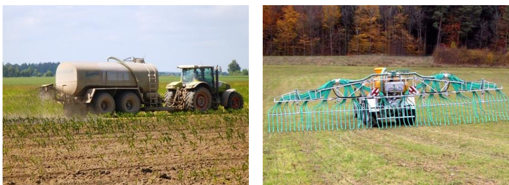
Figure 2-22. Slurry tanker spreading with a splash plate (left) and trailing hoses mounted on a boom (right).
