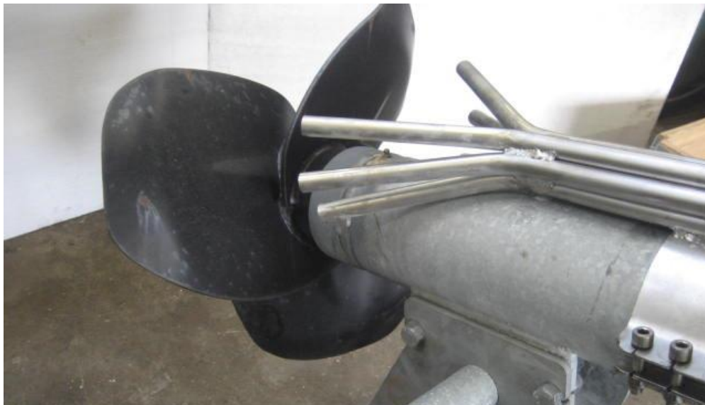
Figure 4.5. Acid delivery system of the Ørum TF-12 slurry acidification system. Photo by Ørum Smeden.
