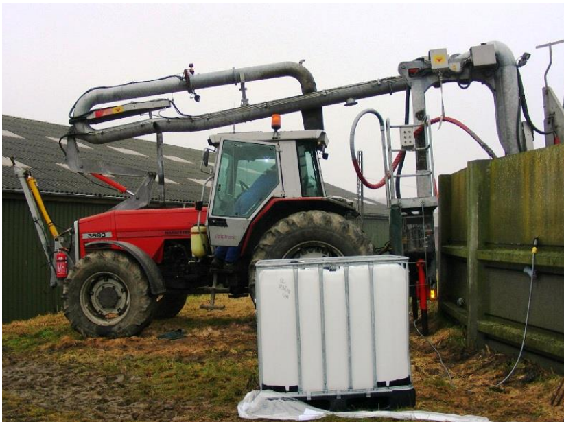
Figure 4.3. The Harsø Compact pump and slurry acidification system. In the foreground is a typical IBC tank used for acid storage. Photo by Harsø Maskiner.
