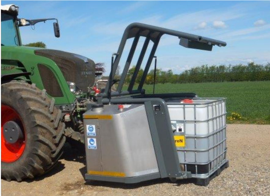
Figure 4.8. The front cage system of SyreN, open during loading of a partially filled IBC tank. The side water tank is also visible. Photo by Biocover.
