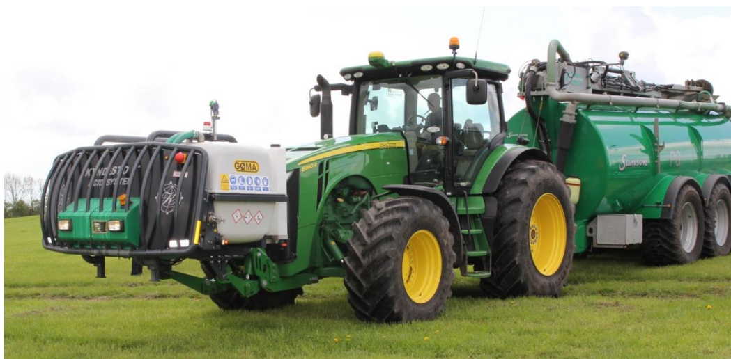
Figure 4.9. Kyndestoft front-tank slurry acidification system.
