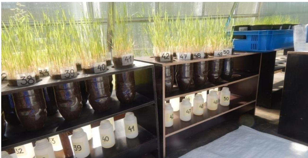
Photo 1. The lysimetric test for slurry (2017).
