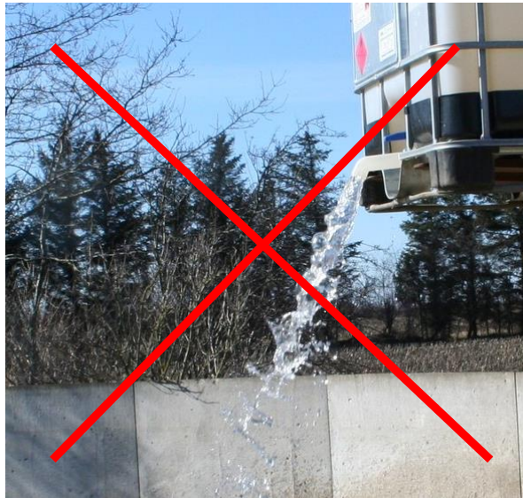
Fig. 3. How not to handle sulphuric acid. Sulphuric acid must not be handled or stored above eye level. http://www.harso.dk/sikkerhed-syre.html
