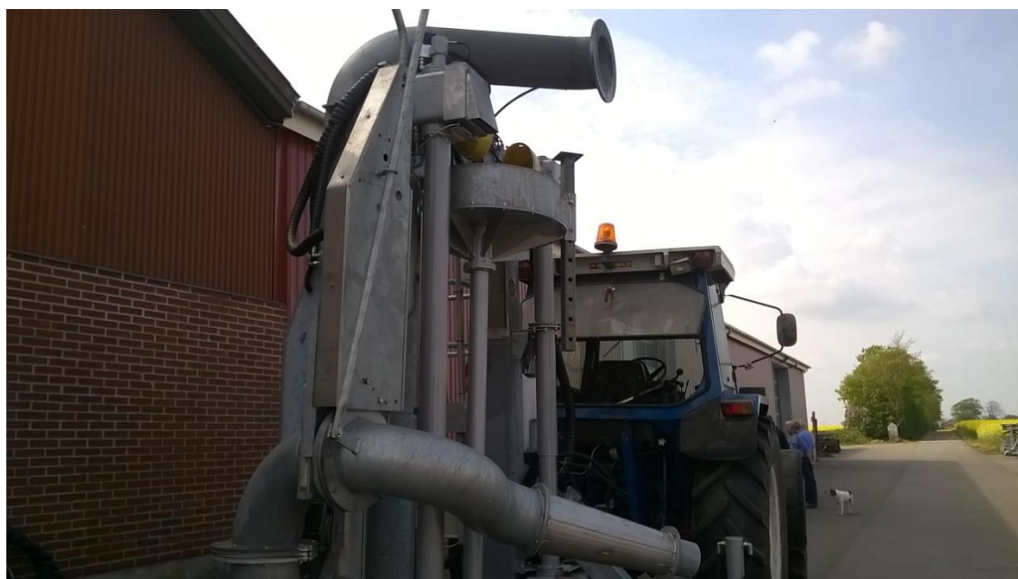
Fig. 13. A system for acidifying slurry in a tank mounted on a tractor.
