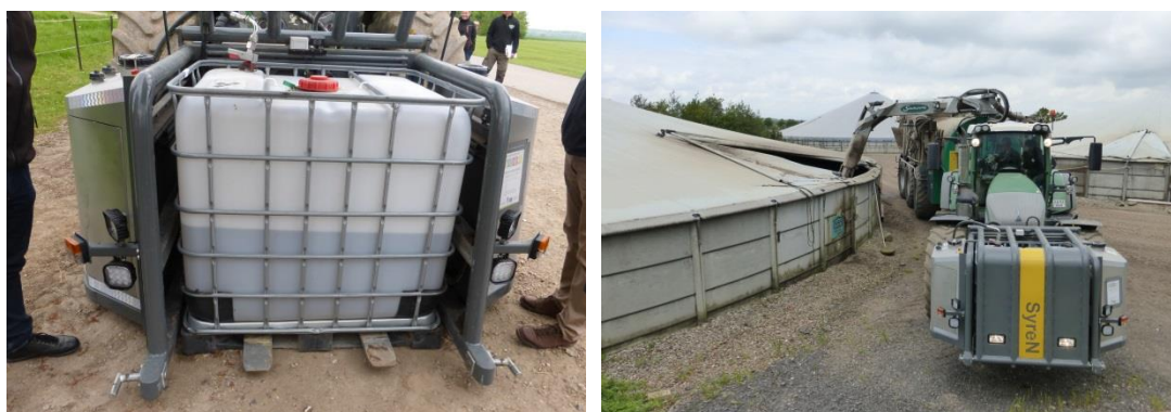
Fig. 6. Mobile intermediate bulk container (IBC) in frame, open (left) and enclosed (right) (made by BioCover A/S).
