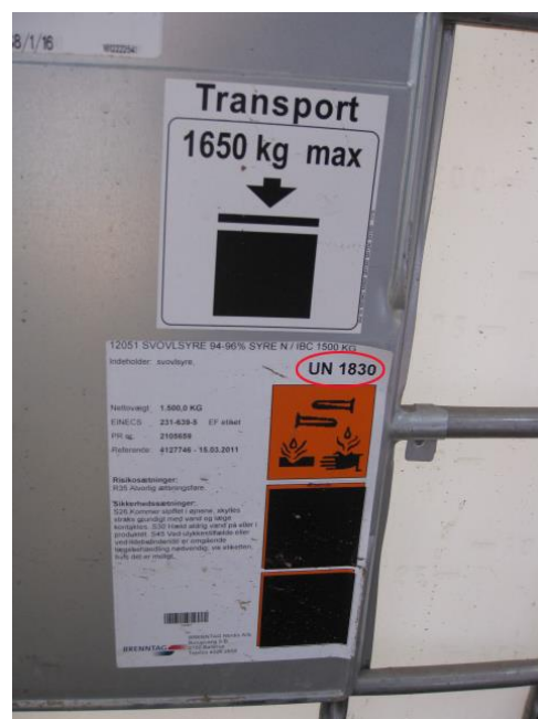
Fig. 9. The UN number for sulfuric acid is UN 1830 (class 8, packing group II).
