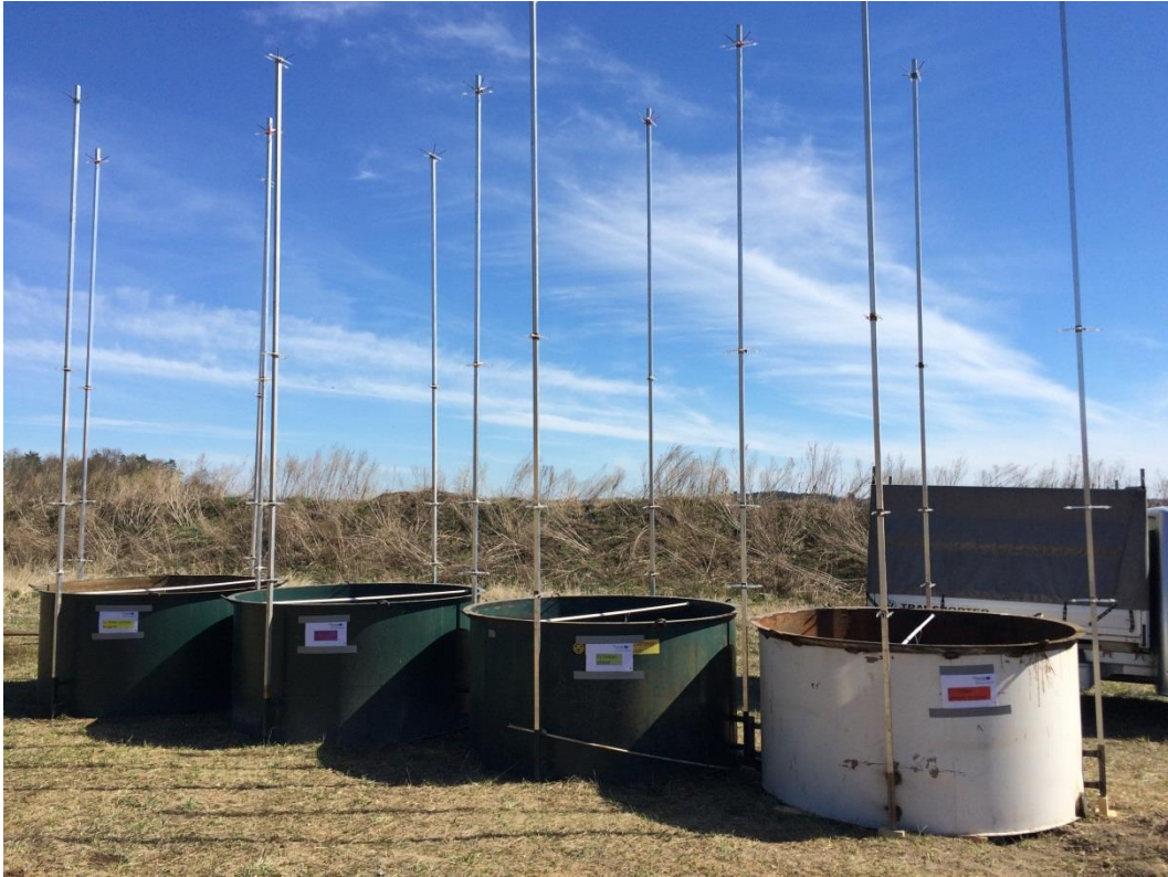
Figure 3. Experimental set up with containers and masts for ammonia measurements with passive flux samplers.
