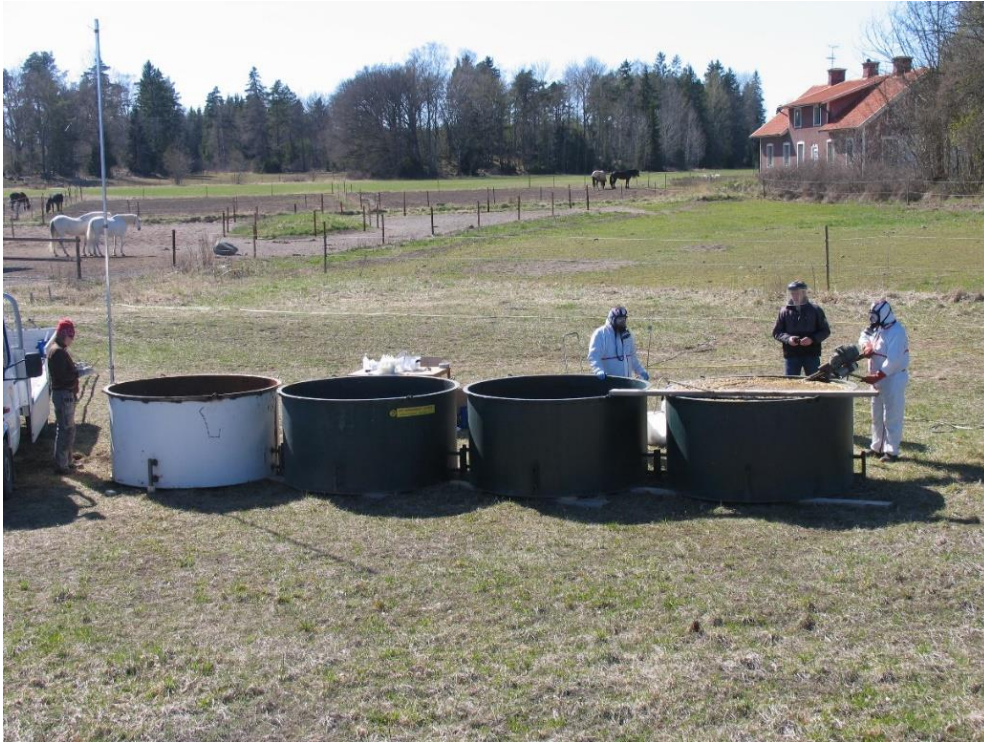
Figure 1. Mixing and addition of sulphuric acid in the storage of DCS (on right). The extensive foaming had to be allowed to settle before more acid was added.
