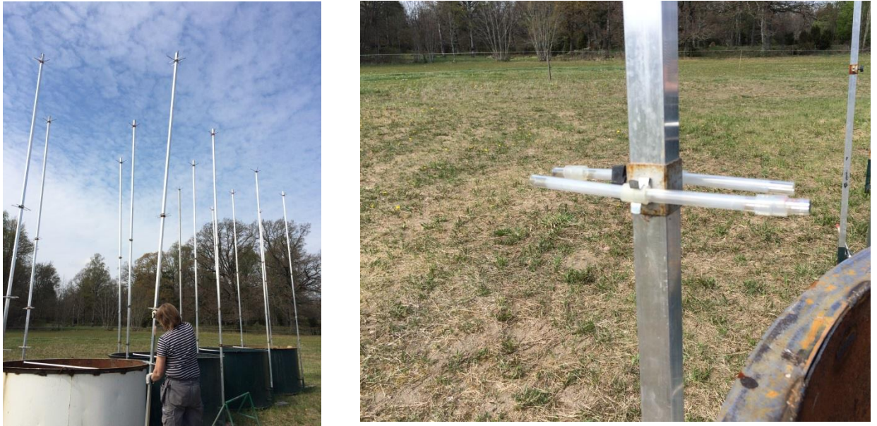
Figure 4. Start of exposure of flux samplers on the second measuring occasion on 18 May (left). Close-up of flux samplers with inlet exposed to the source of ammonia (the slurry) and to the background (surrounding area) (right).
