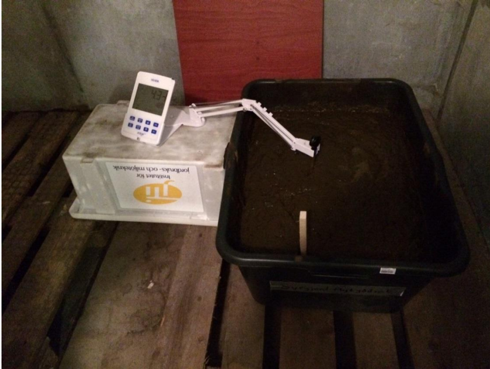
Figure 3. Measuring pH in container with acidified slurry to follow buffering before starting exposure of concrete samples at pH < 5.5 .
