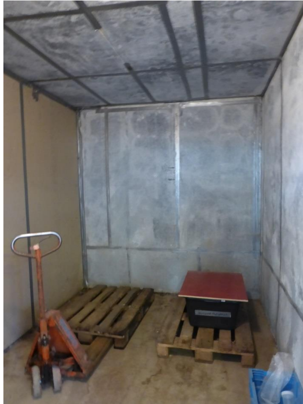
Figure 2. Room with constant temperature 20 °C for exposure of concrete samples to acidified and non-acidified cattle slurry. In the figure the container with acidified slurry and concrete samples is placed in the room and fitted with a non-airtight cover.
