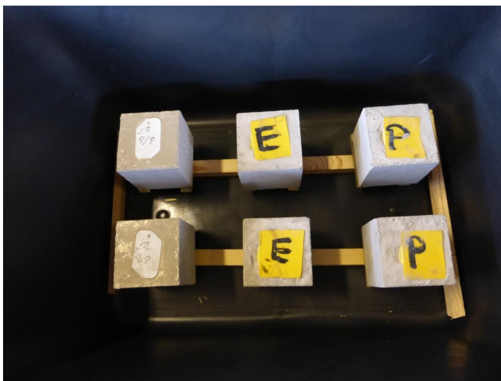
Figure 1. Concrete samples, Sweden. Left: Long lasting concrete; P, concrete in basic platform; E, concrete in wall elements. The samples are placed on a wooden frame made of 20 mm x 20 mm strips at the bottom of a plastic container. During exposure the labels were on the bottom. Samples were placed randomly in each box.
