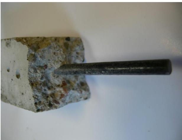
Fig. 40. Condition of the reinforcing bar with a 17 mm cover.
