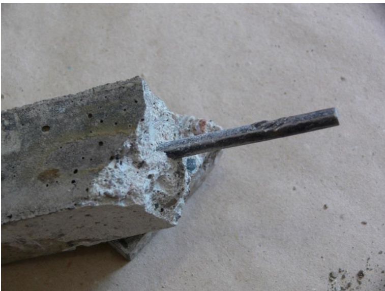
Fig. 62. The sample after bending test. Cover 7 mm. Environment – acidified slurry
