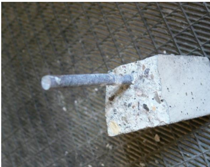
Fig. 50. The sample after bending test. Cover 2 mm. Environment – acidified slurry
