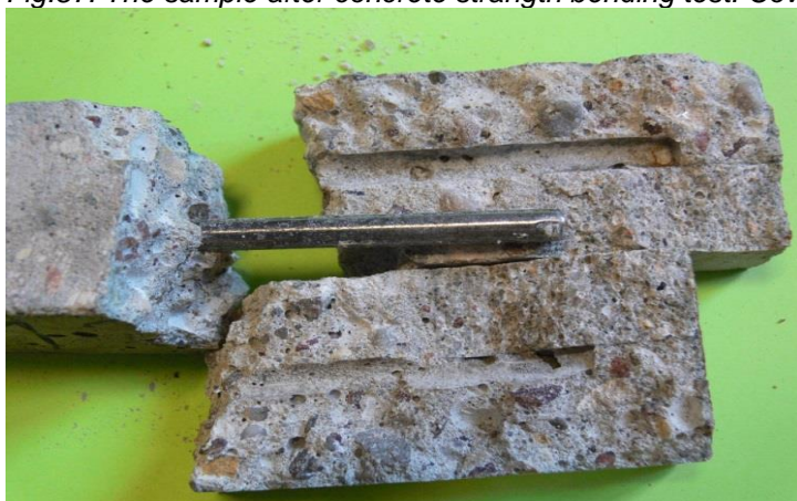
Fig.87. The sample after concrete strength bending test. Cover 7 mm. Environment - acidified slurry
