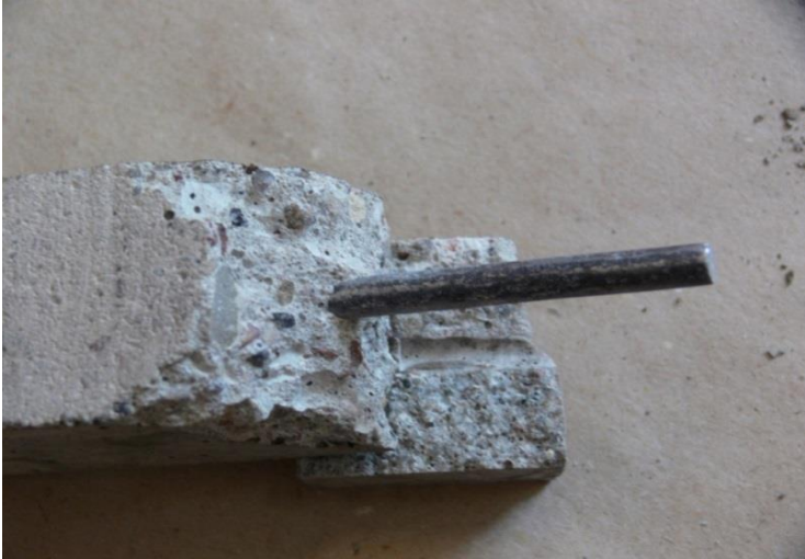
Fig. 60. The sample after bending test. Cover 17 mm. Environment – slurry
