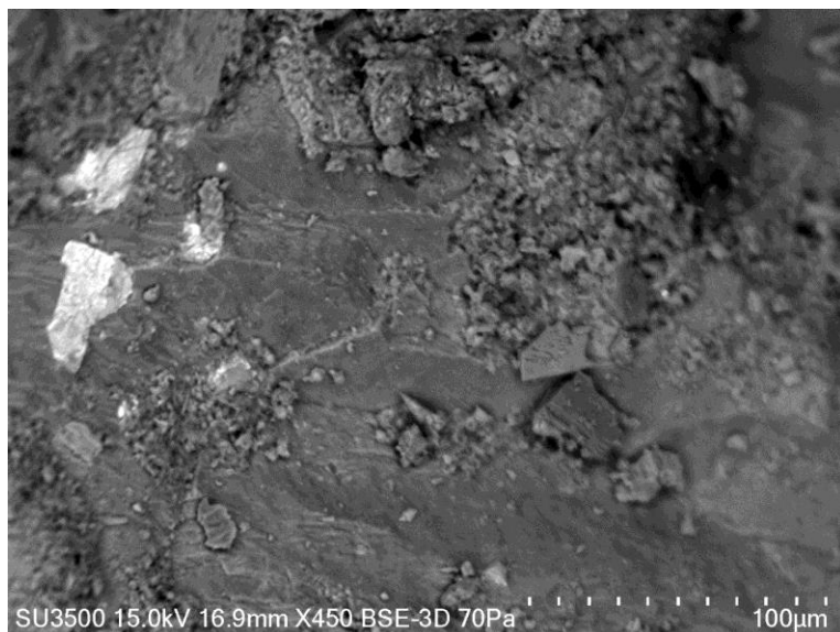
Fig. 95. The bright area - the clusters of iron, titanium with traces of manganese in the concrete of the class C 25/30
