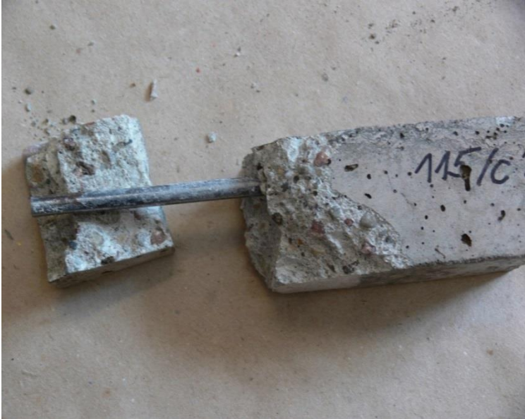
Fig. 62. The sample after bending test. Cover 7 mm. Environment – acidified slurry
