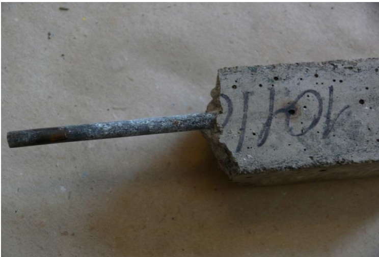
Fig.61 The sample after bending test. Cover 2 mm. Environment – acidified slurry
