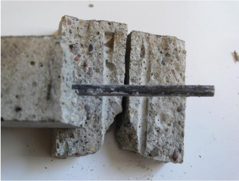
Fig.75. The sample after bending test. Cover 7 mm. Environment – slurry
