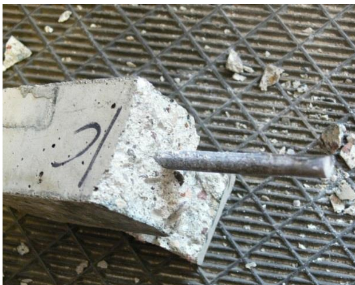
Fig. 52. The sample after bending test. Cover 17 mm. Environment – acidified slurry
