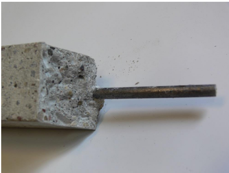
Fig.69. Concrete sample after bending strength test. Side view of the sample
