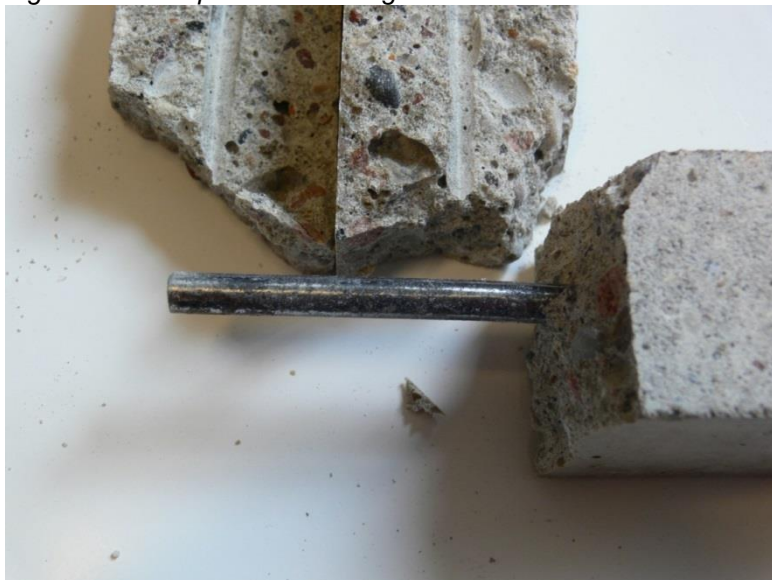
Fig.71. The sample after bending test. Cover 7 mm. Environment – water
