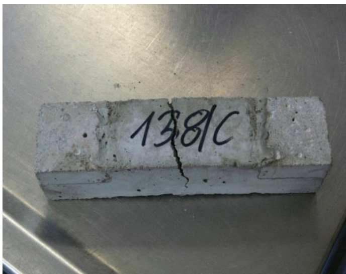
Fig. 37. Concrete sample after bending strength test. Side view of the sample
