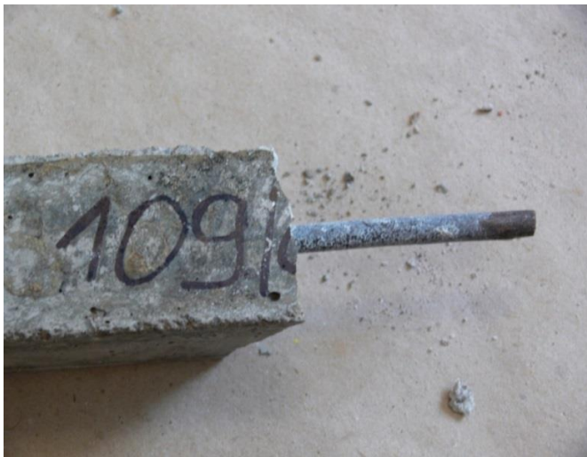
Fig. 58. The sample after bending test. Cover 2 mm. Environment – slurry
