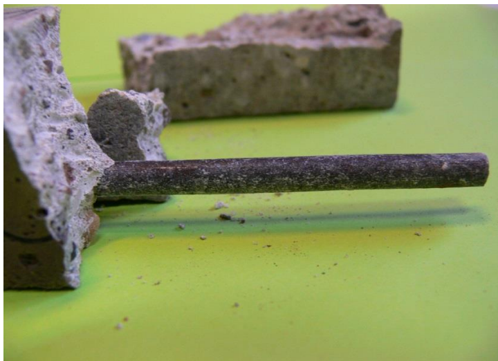
Fig.87. The sample after concrete strength bending test. Cover 7 mm. Environment - acidified slurry
