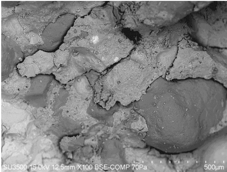
Source: University of A.Mickiewicz Foundation in Poznan ZUB/S/16/12/2018 Fig. 126. Aggregate in a sample of concrete C 25/30
