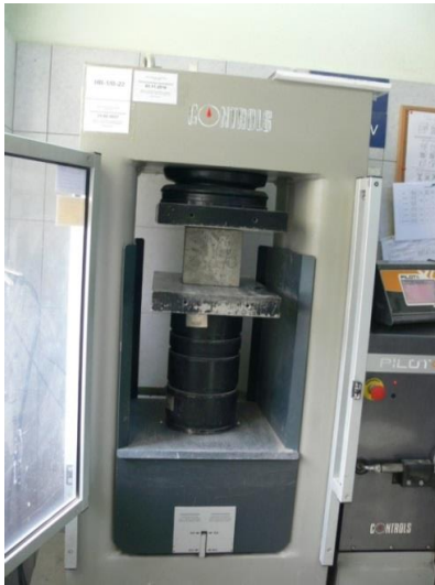
Fig.21. Hydraulic press for compressive strength testing of concrete.
