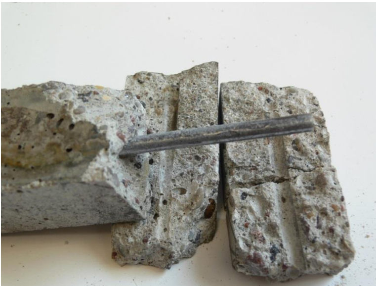
Fig.76. The sample after bending test. Cover 17 mm. Environment – slurry
