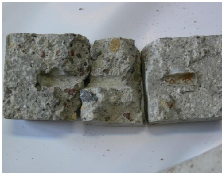
Fig. 41. Recess in concrete, trace of the rod without corrosion
