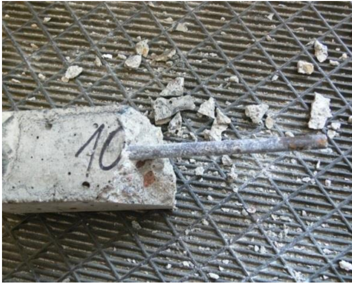
Fig. 50. The sample after bending test. Cover 2 mm. Environment – acidified slurry
