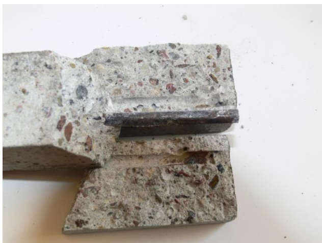
Fig.79. The sample after bending test. Cover 7 mm. Environment – acidified slurry
