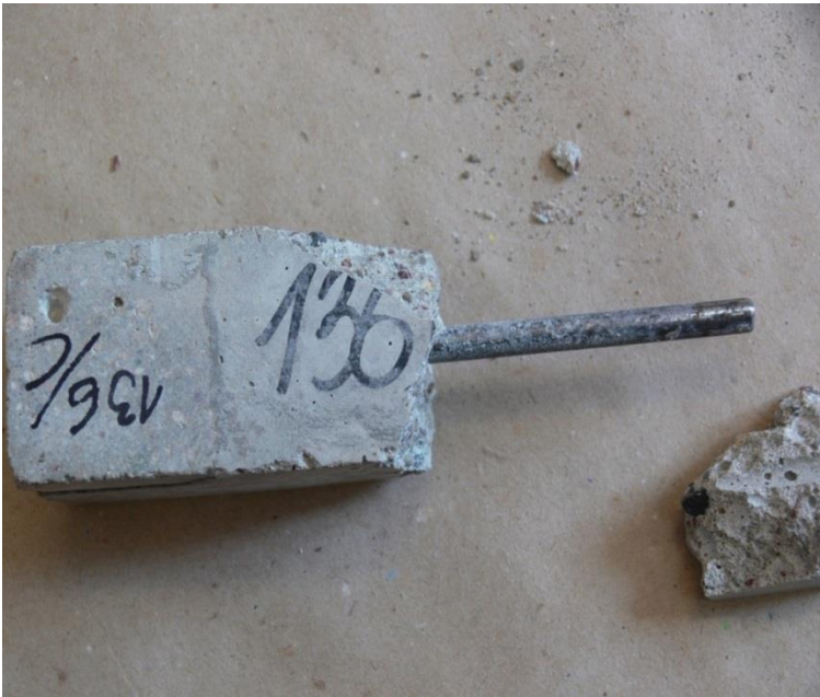
Fig. 56. The sample after bending test. Cover 7 mm. Environment – water
