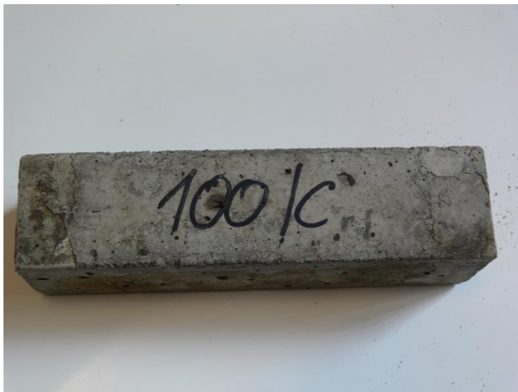
Fig.73. The sample after bending test. Environment – slurry
