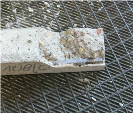
Fig. 44. The sample after bending test. Cover 2 mm. Environment – water
