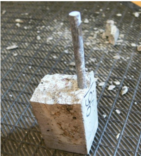
Fig. 47. The sample after bending test. Cover 2 mm. Environment – fresh slurry
