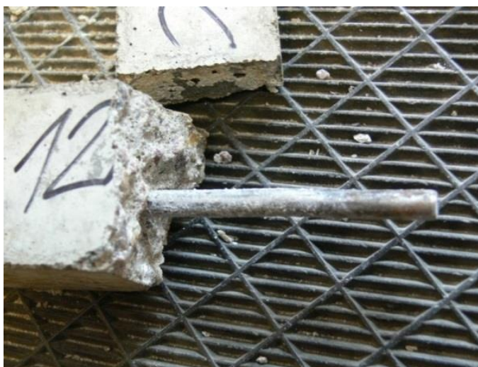
Fig. 49. The sample after bending test. Cover 17 mm. Environment – fresh slurry
