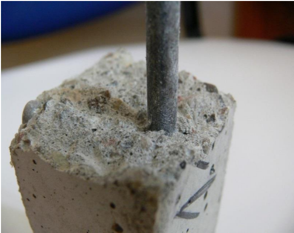
Fig. 39. Condition of the reinforcing bar with a 7 mm cover.
