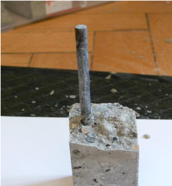
Fig. 44. The sample after bending test. Cover 2 mm. Environment – water
