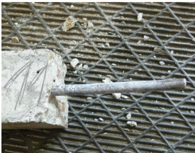
Fig. 48. The sample after bending test. Cover 7 mm. Environment – fresh slurry
