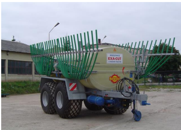
Fig. 10. Plastic slurry tanker with trailing hoses.
