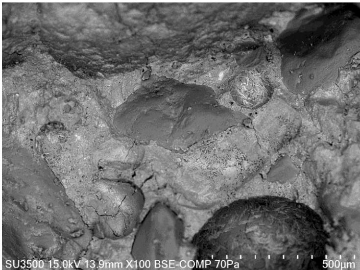
Fig. 103. The bright areas are the forming of etryngite crystals in C 30/37 concrete in a hollow after the removal of the aggregate / top and bottom of the photo / grain.
