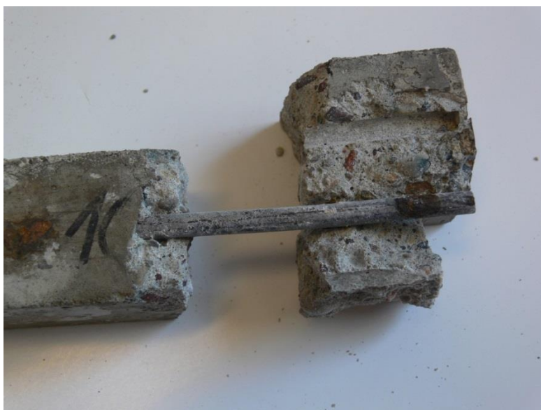
Fig.78. The sample after bending test. Cover 2 mm. Environment – acidified slurry
