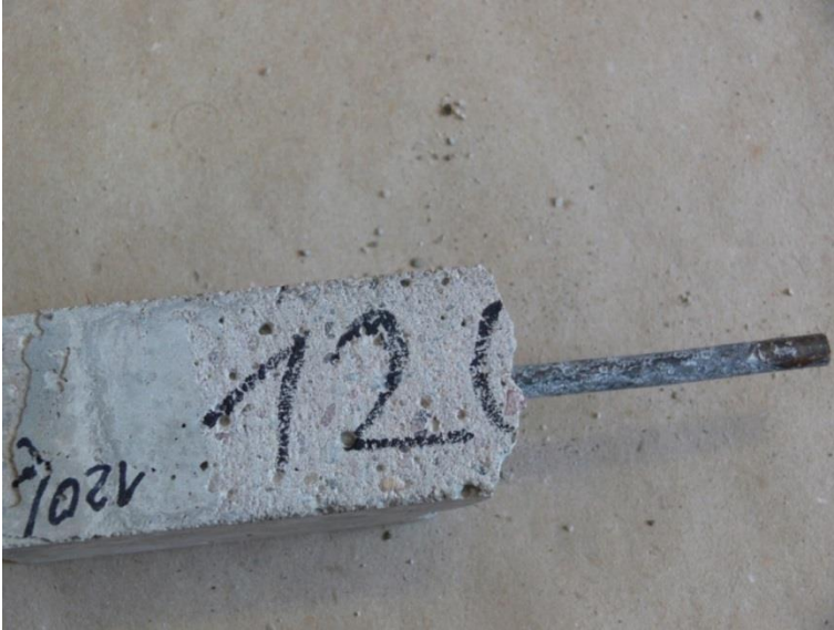
Fig. 56. The sample after bending test. Cover 7 mm. Environment – water
