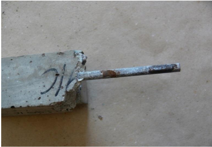
Fig. 58. The sample after bending test. Cover 2 mm. Environment – slurry
