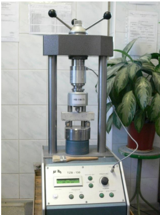
Fig. 32. Press with an attachment for testing the bending strength of concrete
