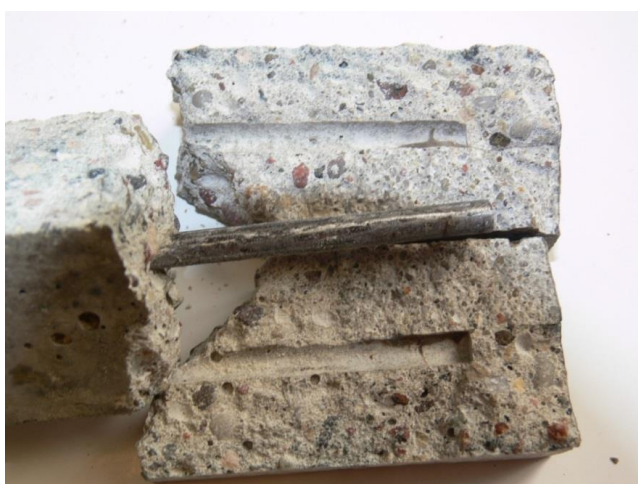
Fig.80. The sample after bending test. Lagging 17 mm. Environment – acidified slurry
