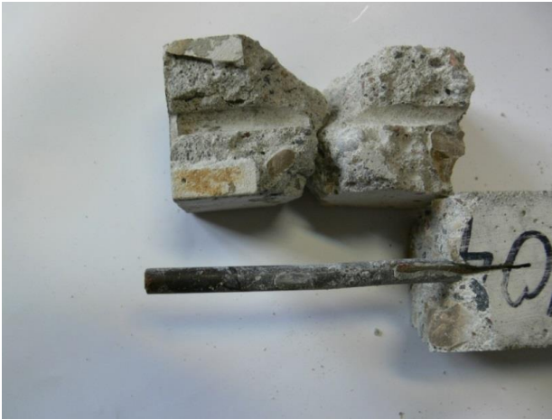
Fig. 38. Condition of the reinforcing bar with a 2 mm cover.
