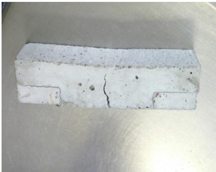
Fig. 36. Concrete sample after bending strength test. Side view of the sample
