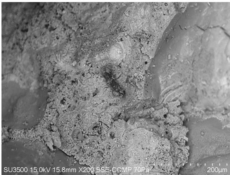
Fig. 123. Small pores in a concrete sample C 25/30 / dark points /
