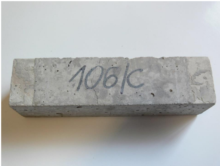
Fig.69. Concrete sample after bending strength test. Side view of the sample
