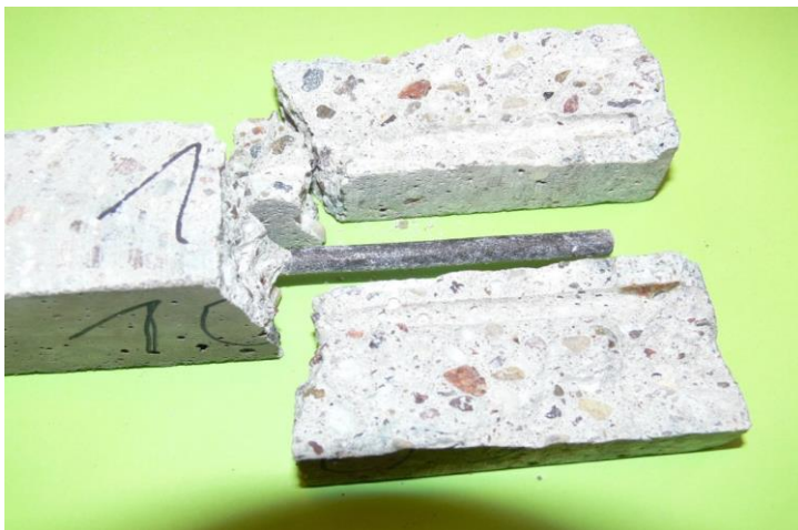
Fig.86. The sample after concrete strength bending test. Cover 2 mm. Environment - acidified slurry
