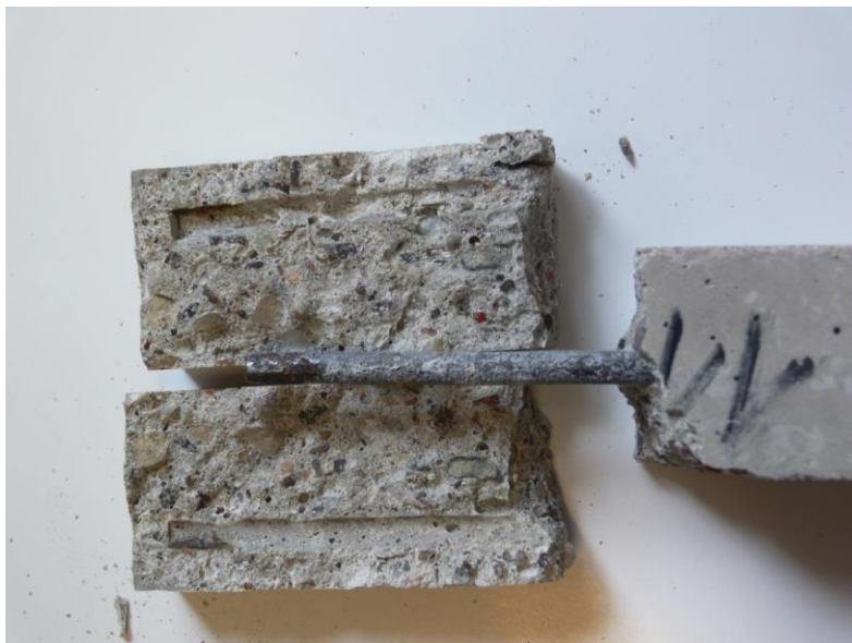
Fig.71. The sample after bending test. Cover 7 mm. Environment – water
