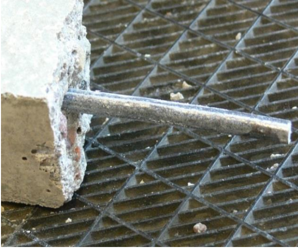
Fig. 46. The sample after bending test. Cover 17 mm. Environment – water
