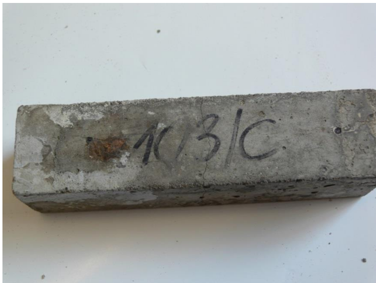
Fig.77. Concrete sample after bending strength test. Environment – acidified slurry
