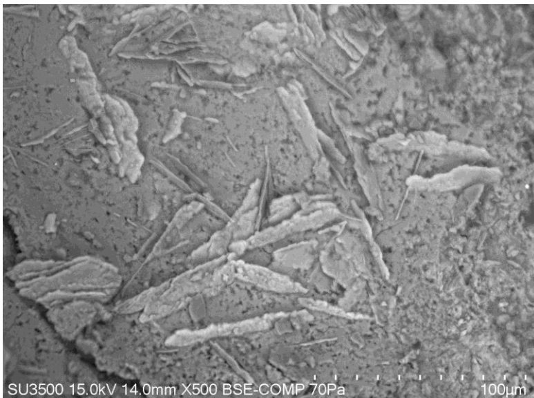
Source: University of A.Mickiewicz Foundation in Poznan ZUB/S/16/12/2018 Fig. 129. The bright areas are the forming of ettringite crystals concrete in C 25/30.
