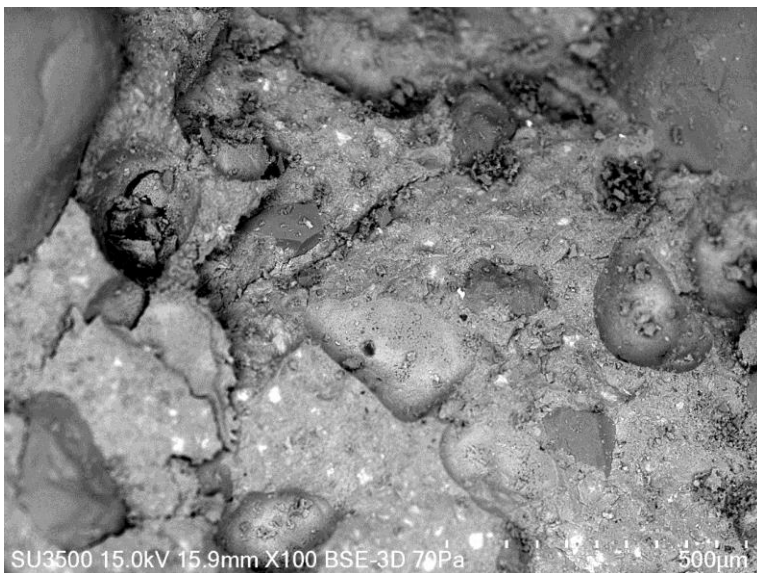
Source: Foundation of A. Mickiewicz University in Poznan WK/S/13/03/2017 Fig.92. Grains of aggregate in a concrete sample of a class C 30/37
