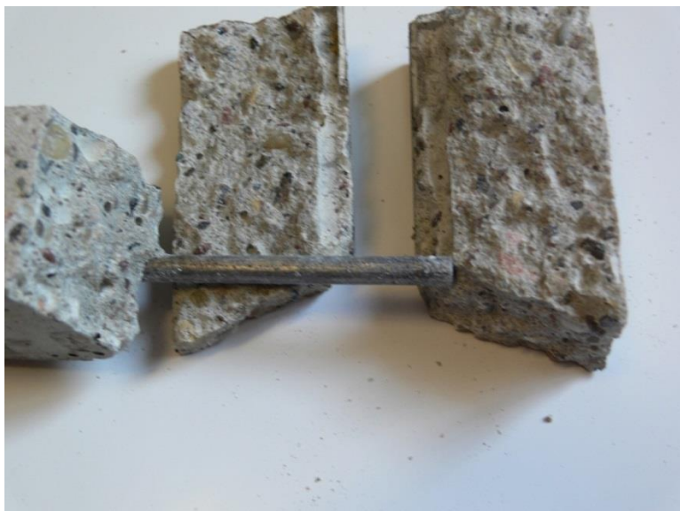
Fig.74. The sample after bending test. Cover 2 mm. Environment – slurry
