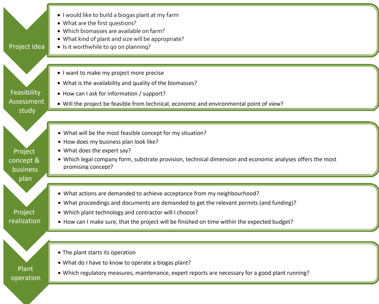
Figure 3. Project development phases and fundamental questions for setting-up a biogas plant
