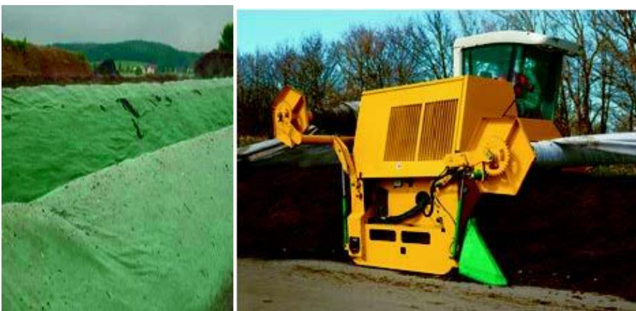
Figure 19: Stack covering with semi-permeable membranes
