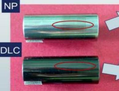
No evidence of wear for coated pin
