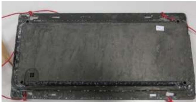
Salt Spray Test in accordo con ASTM B117-07
