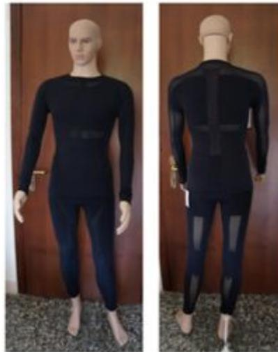
Figure 3 Sensor suit prototype
