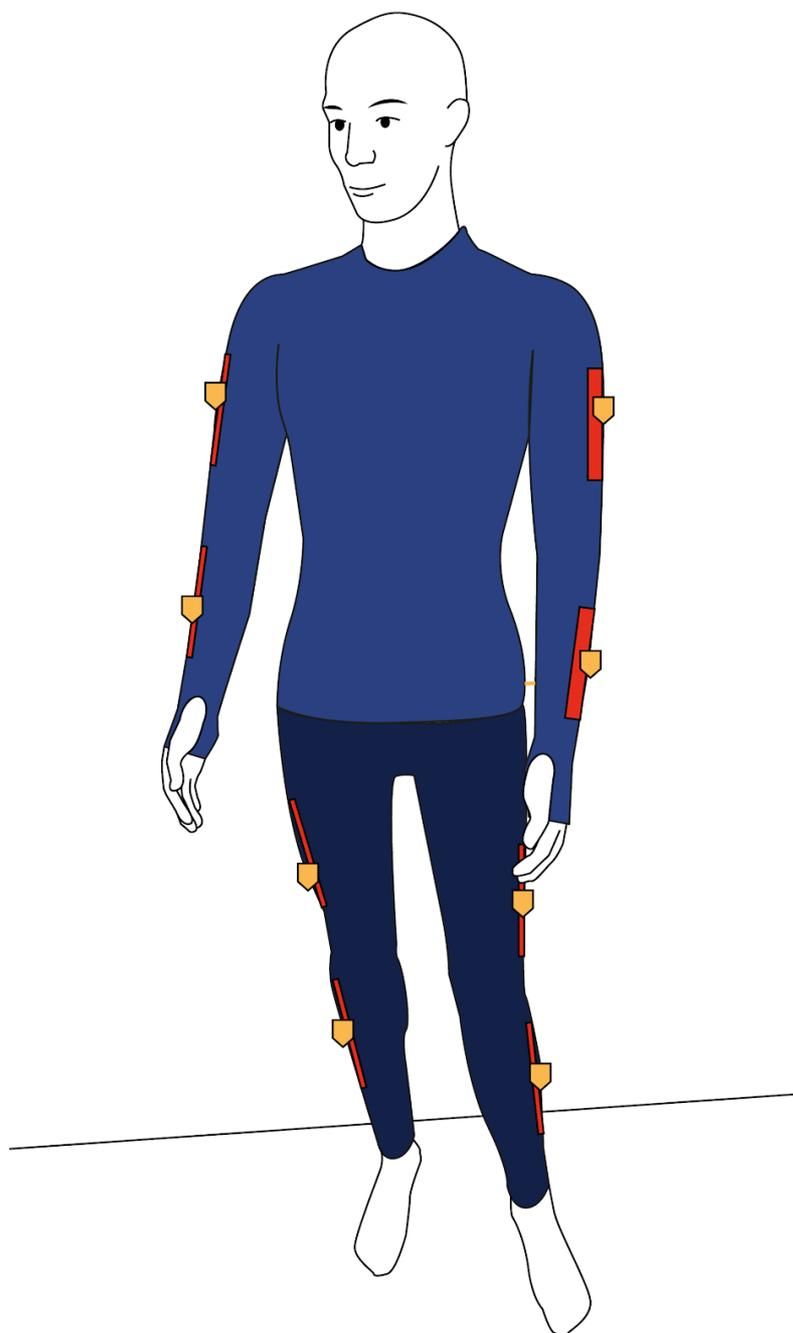
*Position of the IMU sensors on the suit*
