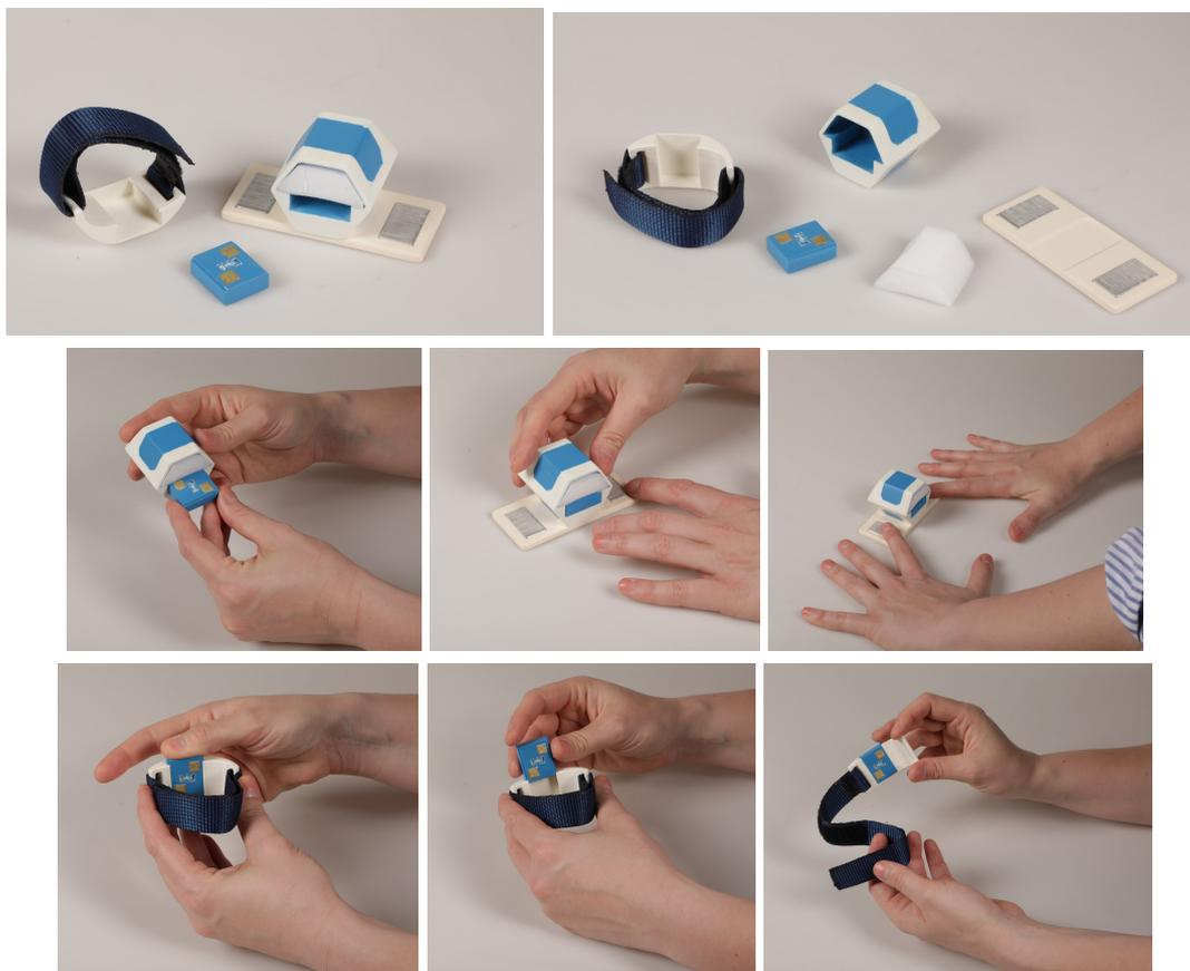
*3D printed models of hub and wristband with removable sensors*
