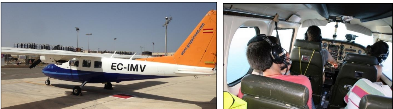
Fig. 13. (Left) Aircraft for monitoring floating macro litter and (Right) crew made by the pilot on the left hand of the plane, data recorder in the seat of the co-pilot, two observers positioned at each side of the plane and an additional observer dedicated to photo shooting.
