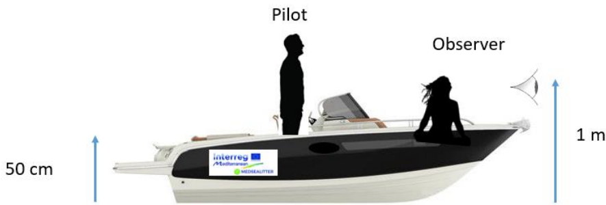
Fig. 4. Small vessel (50 cm above sea surface) with an observation height of ~ 1 m.
