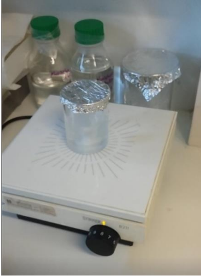
Fig. 38. Dilution and homogenization process over magnetic stirrer.
