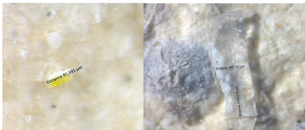
Fig. 49. Detected microplastic images measured by mean of image analysis software.
