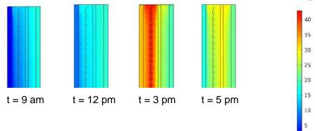
Figure 10: Temperature distribution within the CFS at different times
