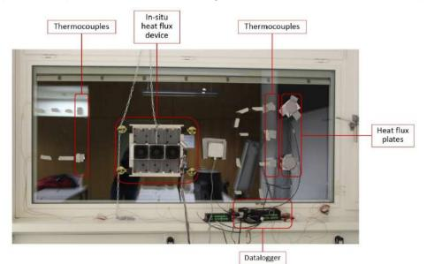
Figure 8: Measurement setup for the CFS
