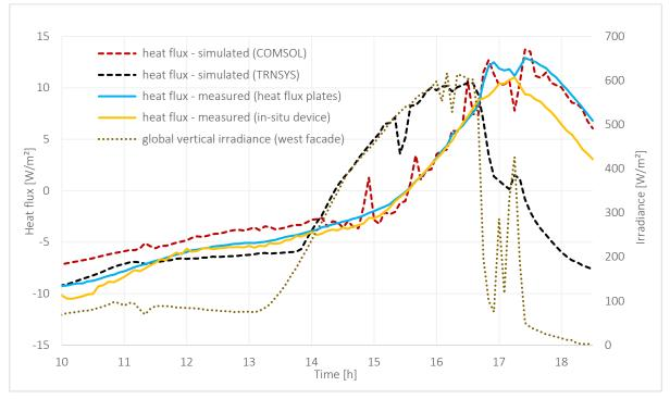
Figure 9: Comparison of simulated and measured heat flux through the CFS.
