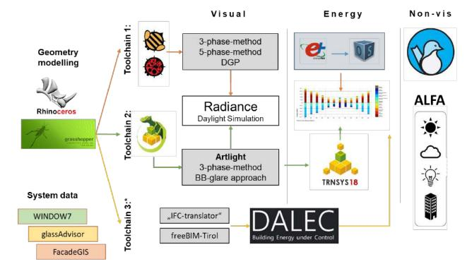
Figure 16: FACEcamp simulation toolchain for complex facade systems
