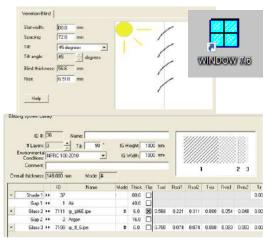
Fig. 2: Glazing + shading system setup in WINDOW7
