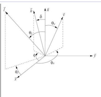
Figure 3: : Diagram showing vectors used to define the BSDF
