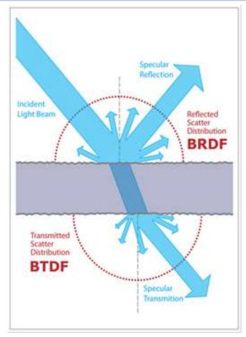
Figure 2: The composition of a BSDF. BSDF = (BTDF + BRDF), BSDF – bidirectional scattering distribution function, BRDF – bidirectional reflection distribution function, BTDF – bidirectional transmission distribution function. (Source: <u>https://en.wikipedia.org/wiki/Bidirectional\_scattering\_distribution\_function</u>)
