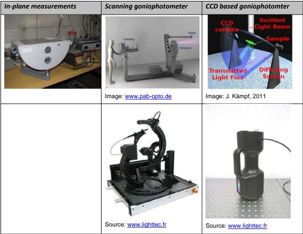
Fig. 3: Methods of BSDF determination by measurements
