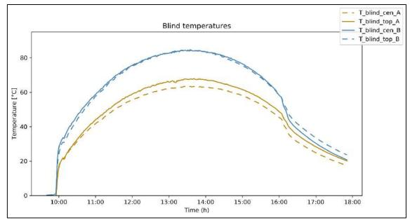
Figure 5: Blind temperatures for the two façade samples on a clear sky day; sensors named "cen" are positioned on a blind at the centre of the window, sensors named "top" are positioned at a distance of ¼ of the total height from the upper limit; closed cavity
