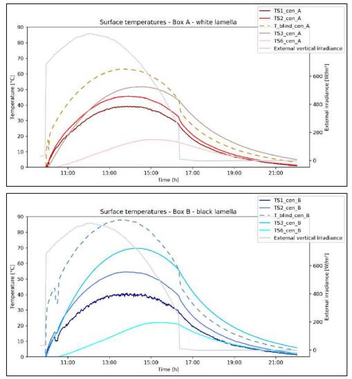
Figure 8: Surface temperatures of façade sample A (top) and B (bottom). Detail of glazing centre-of-glass surface and blinds temperatures. Open cavity configuration. TS1 = face 1, TS2 = face 2, TS3 = face 3, TS6 = face 6. (Face 4 and 5 are the internal faces in the IGU).
