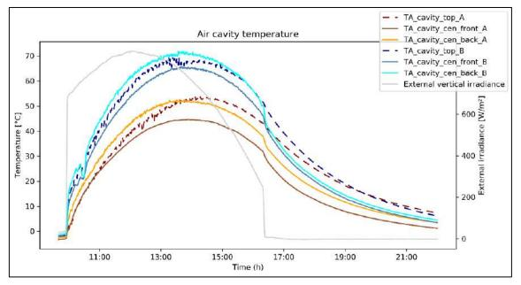
Figure 10: Air cavity temperatures for façade sample A and B – open cavity.
