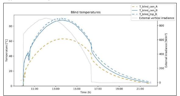
Figure 6: Blind temperatures for the two façade samples on a clear sky day; sensors named "cen" are positioned on a blind at the centre of the window, sensors named "top" are positioned at a distance of ¼ of the total height from the upper limit; open cavity.
