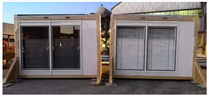
Figure 2: Front view of the two façade samples, right: sample A with externally white blinds, left: sample B with externally black blinds.
