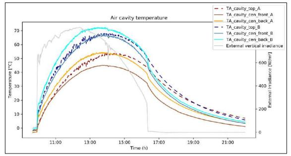
Figure 9: Air cavity temperatures for façade sample A and B – closed cavity
