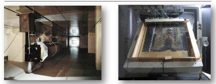
Figure 6: top: whole test stand, bottom-left: solar simulator, bottom-right: probe fixture in the climatic chamber
