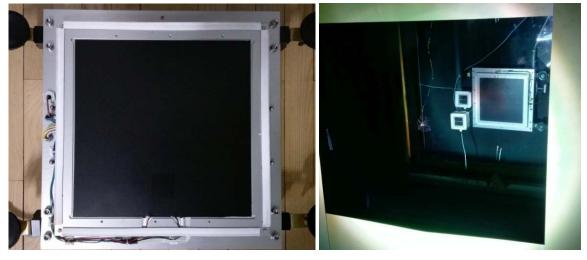
Figure 8: Prototype with absorbing foil (L) installation in calorimetric test stand at BB (R)
