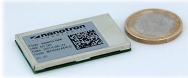
Figure 5: CSS PHY radio module by Nanotron Technologies® [39].
