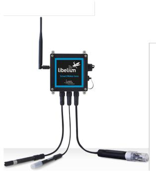
Figure 13: The Libellium® smart sater end-node, implementing the LoRAWAN specification for monitoring water quality parameters.
