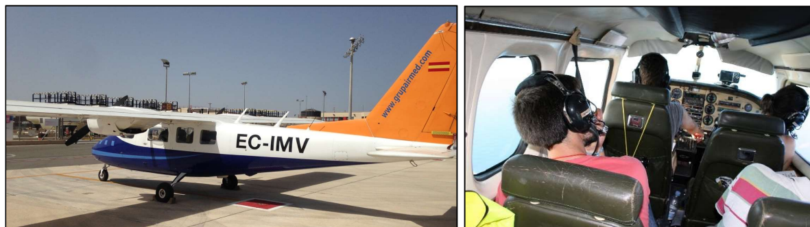
Figure 2 (a) Aircraft for monitoring floating macro litter and (b) crew made by the pilot on the left hand of the plane, data recorder in the seat of the co-pilot, two observers positioned at each side of the plane and an additional observer dedicated to photo shooting.
