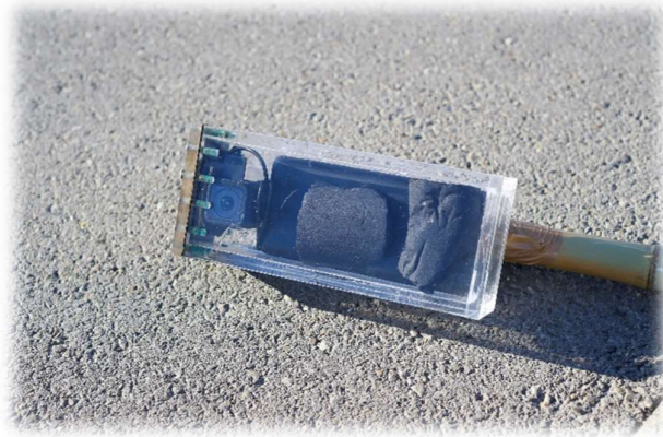
Figure c. Polarized GoPro Hero Session camera combined with an Anker PowerCore 26800 external battery, protected in Homemade waterproof Plexiglas box.
