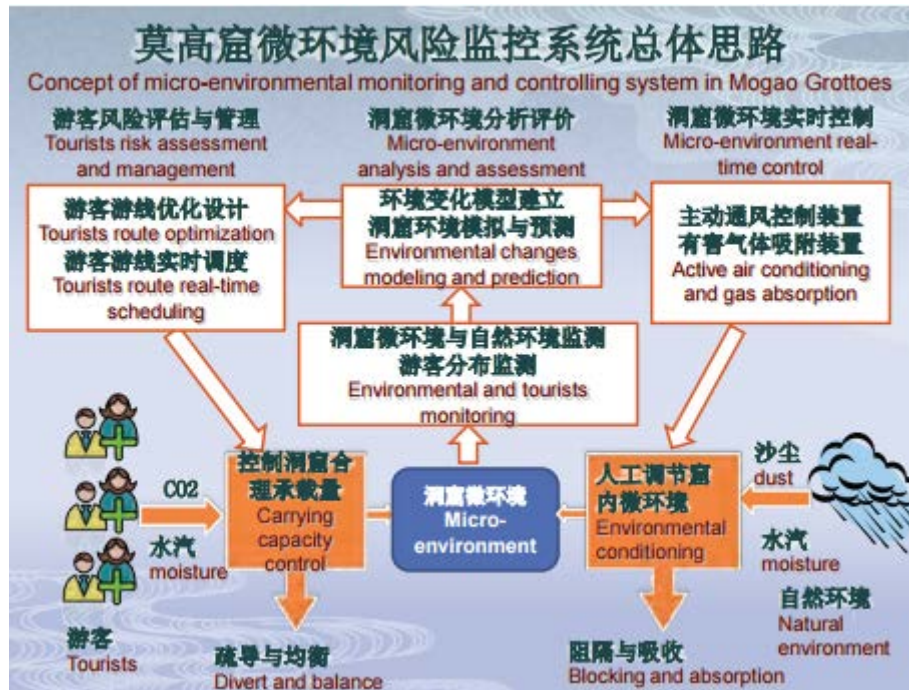
Figure 7 - Structure of Micro-environmental monitoring and controlling system in Mogao Grottoes (China)
